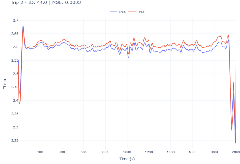
(a) Predictions for the easier test trip ( V(\theta) = 2.45 ). We see that the prediction overshoots slightly at most points, but that the overall pattern is captured well.
