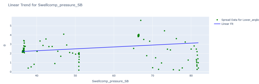
Figure 36: Data does not seem to follow the trend that well. There are also no data points in between 50 and 70 on the x axis.
