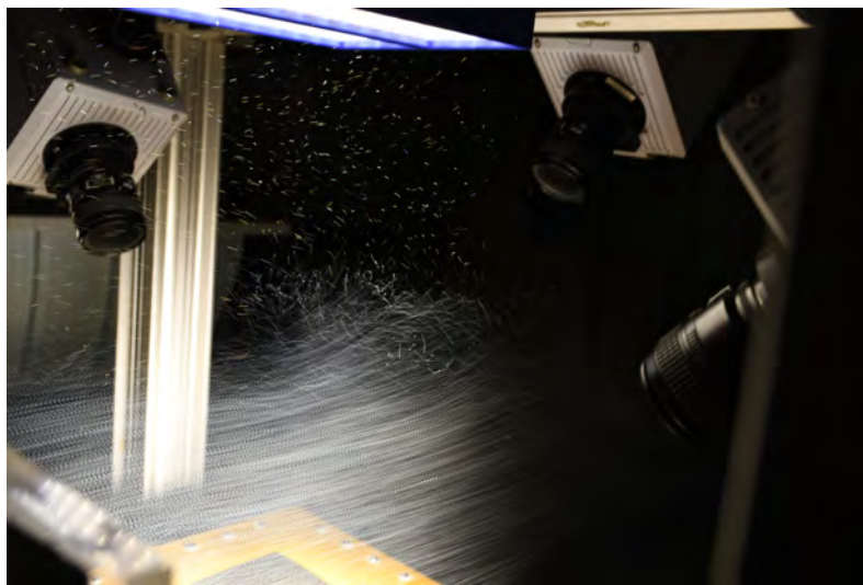
Figure 6.2: Experimental setup in operation with HFSB illuminated by means of the three LED light sources.
