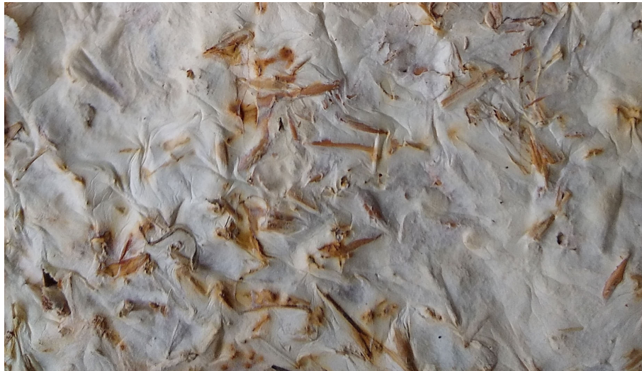
FIG. 6.5 Mycelium-fibre insulation panel [Source: Bob Geldermans]
