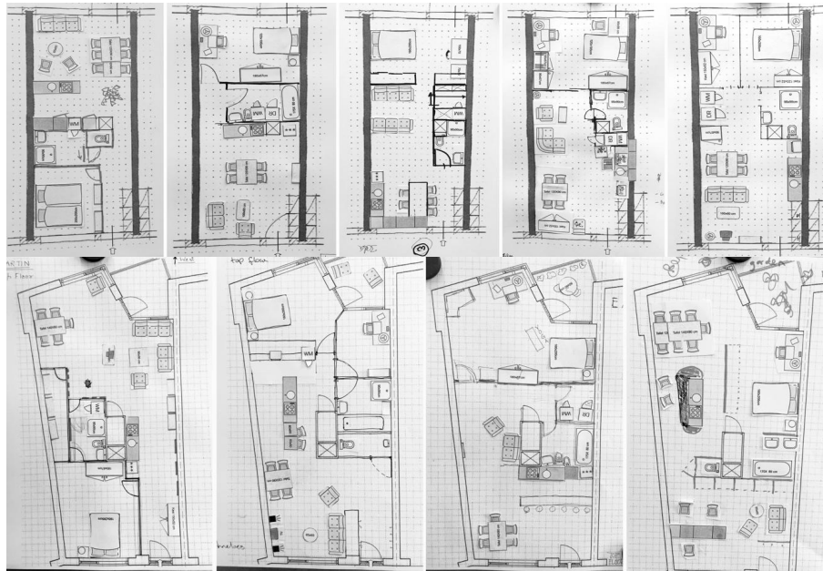
FIG. 4.6 Results from the workshop. Above, five floor-plans of dwelling type 1 (50 m 2 ). Below, four floor-plans of the dwelling type 2 (70 m 2 ) [Source: Bob Geldermans and Frans van der Werf]
