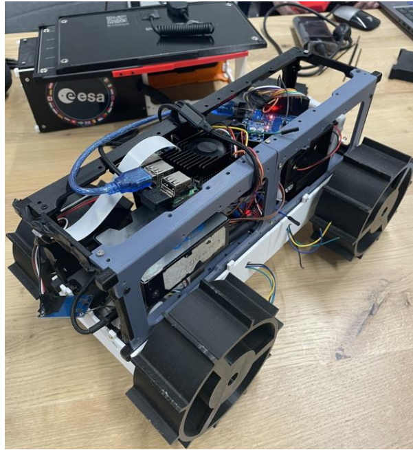
Figure 17: Mock-up CubeSat-based rover structure assembly
