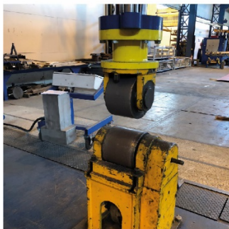
'English wheel' using Roll Forming
