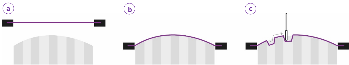
Figure 47: Used production method for creating sandwich panels, a combination between Stretch Forming and Incremental Sheet Forming.
