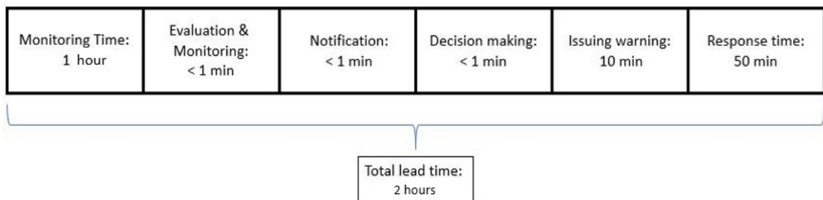
Figure 6.3: Lead time required by the BRT-system
