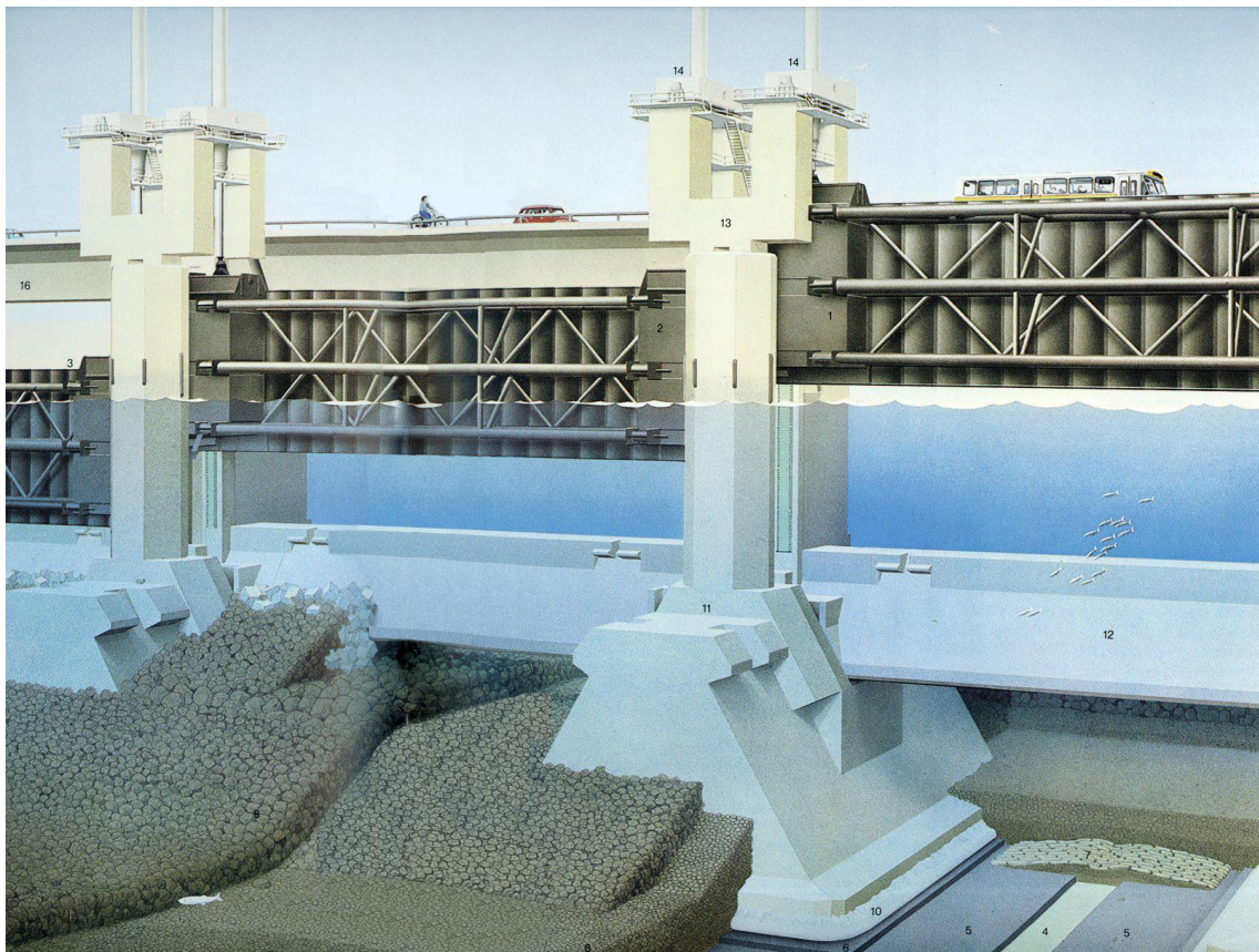
Figure 20: threshold of the barrier
