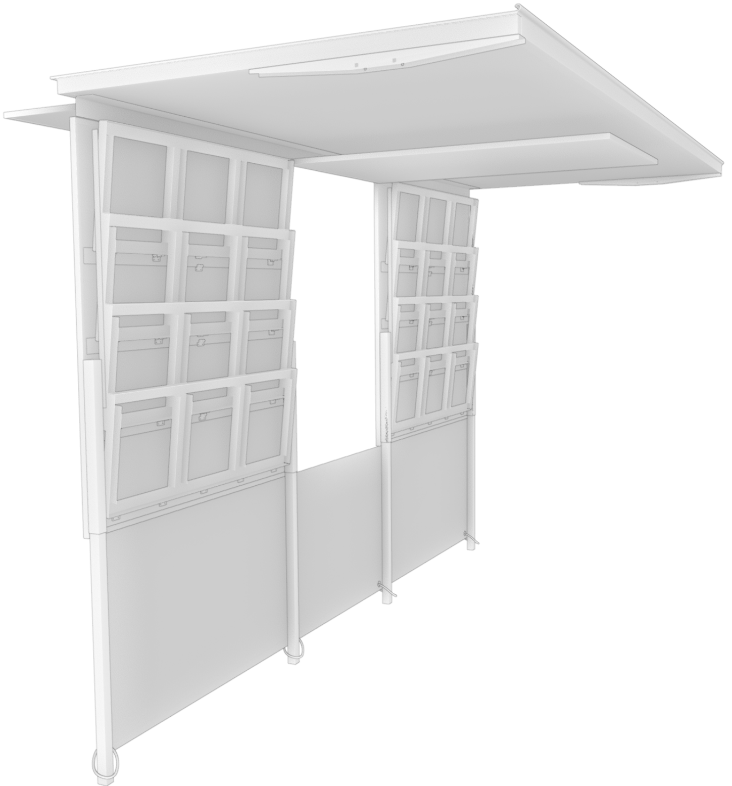
Side panel with all shelves collapsed, and the middle section opened
