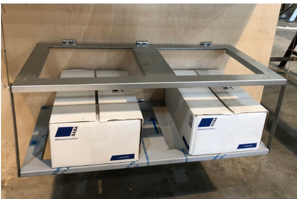
Third test, performed by InnovaN; Testing deformation with a mass of 30kg
