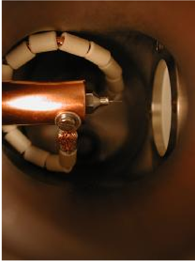
Figure 2: Field emission microscope. The figure shows the emitter tip (left side) and the screen (right side).
