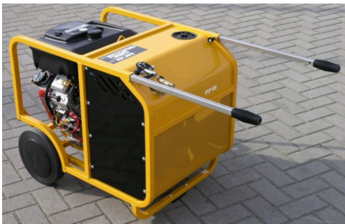
Figure I.3: The PP018 Hydraulic Power Unit (Sub. Ind., 2018)
