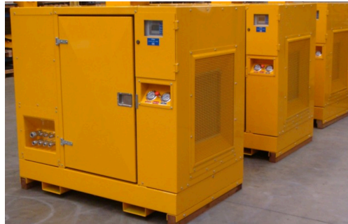
Figure I.4: The PP100 Hydraulic Power Unit (Sub. Ind., 2018)
