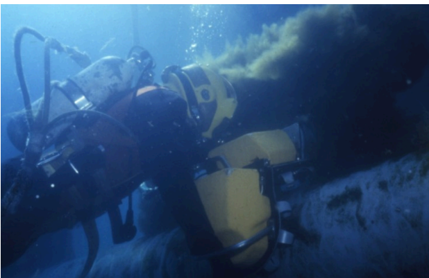
Figure H.3: Working with The Twin Brush Unit (Subsea Industries, 2018)
