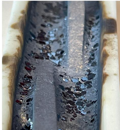
**Figure B-3:** Preliminary experiment of copper oxide infiltration in an alumina porous body, showing crystal formation on the surface
