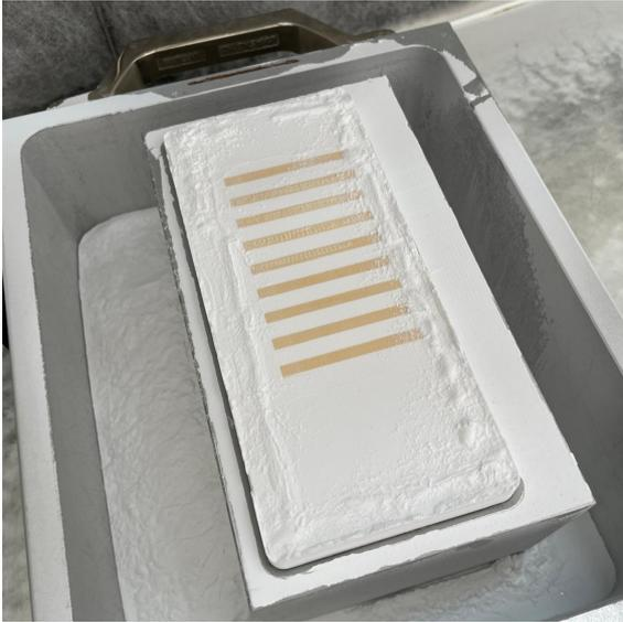
**Figure 3-3:** Cured alumina bending bar samples produced by PBBJ embedded within the powder bed
