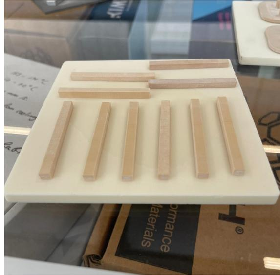
**Figure 3-4:** Cured alumina bending bar samples produced by PBBJ depowdered and put onto a alumina flat plate
