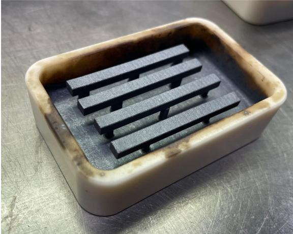
**Figure 4-6:** infiltrated sample bending bars still attached to infiltration setup, infiltrated in an oxygen rich environment
