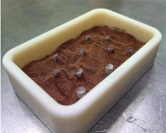
**Figure 3-10:** Infiltration setup B, with powder along the infiltration pillars
