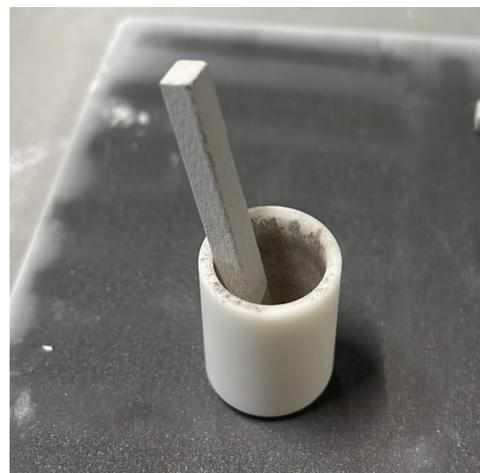
**Figure 3-7:** Infiltration setup A before the pressureless infiltration
