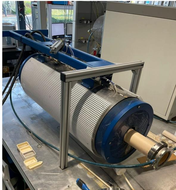
**Figure 3-12:** Lenton tube furnace, used for infiltration
