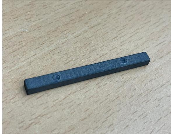
**Figure 4-7:** Image of a detached bending bar sample that was previously attached to the infiltration setup B. The broken joints are visible in the figure
