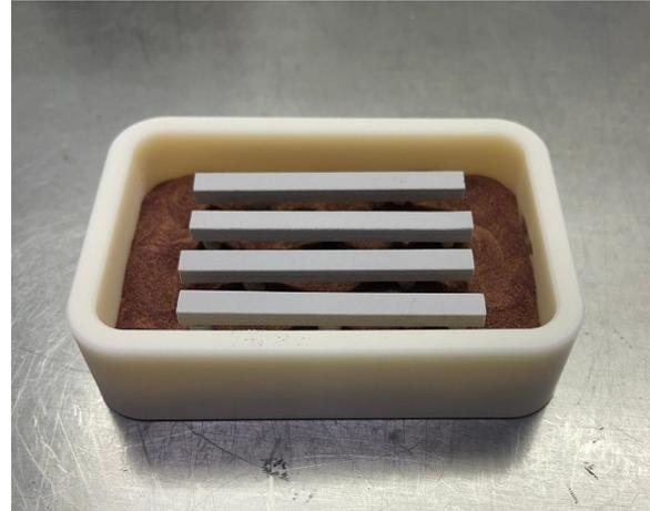
**Figure 3-11:** Infiltration setup B, with the bending bar samples on top of the infiltration pillars
