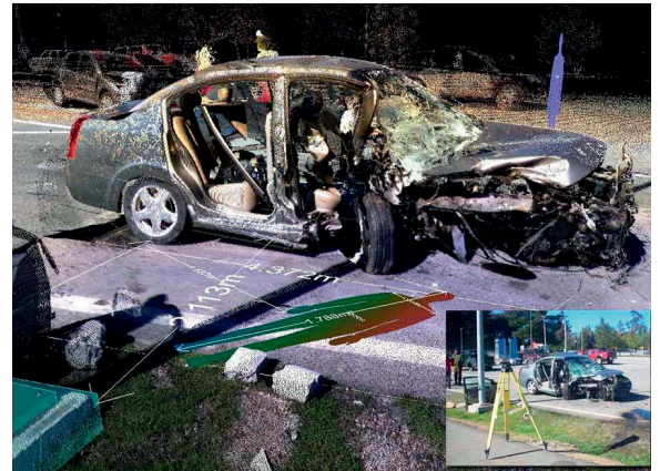
▲ Figure 2, Analysed point cloud of a crash site captured by TLS (courtesy of Maptek).
