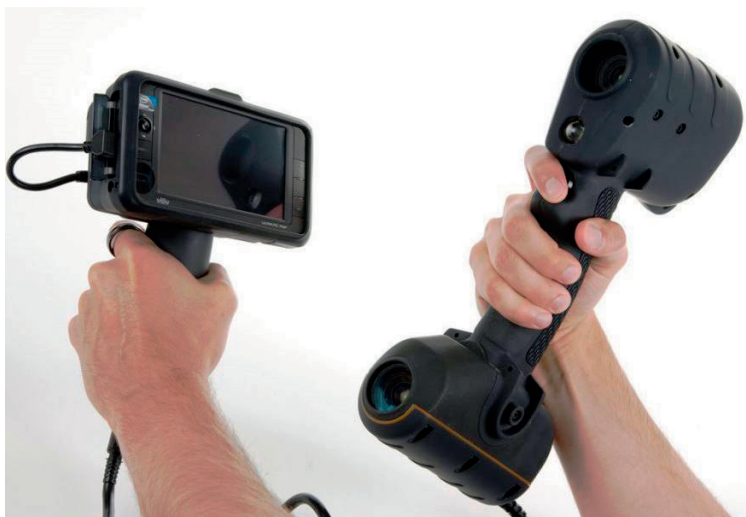
▲ Figure 3, The Mantis Vision F5 handheld laser scanner weighs 1.7kg and has a range of 4.5m.
