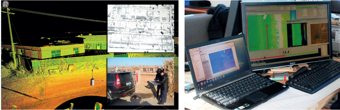
▼ Point cloud of a village in the Heilongjiang province in China captured by RIEGL VZ-400 for cadastral purposes.
