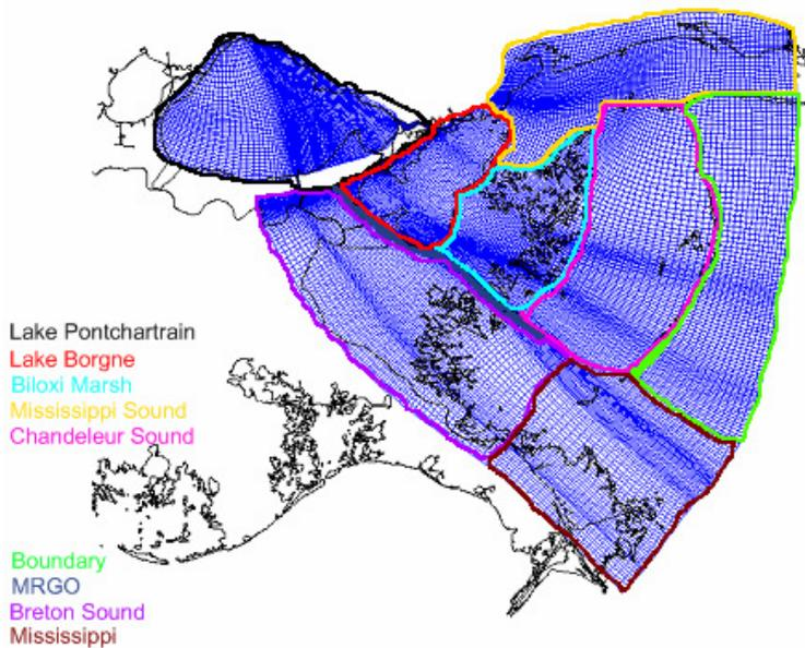
Figure 7.6 Sections in tracer analysis
