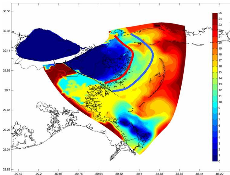
Figure 7.11 The 10 ppt and 15 ppt isohaline for the diversion scenario
