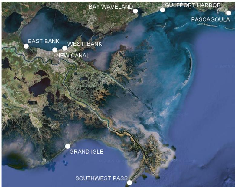
Figure 4.21 Location of gages used in ADCIRC storm surge modeling (Google Earth, 2009)
