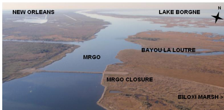
Figure 4.2 Rock dam as closure of the Mississippi River Gulf Outlet (MRGO) at Bayou La Loutre
