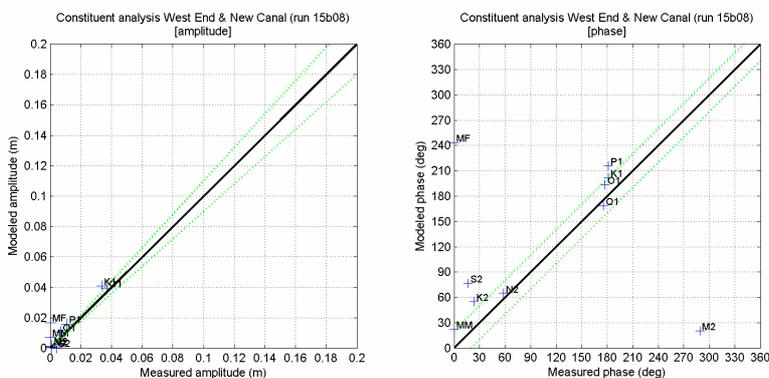
Figure 5.16 Constituent analysis New Canal (West End) (calibrated)
