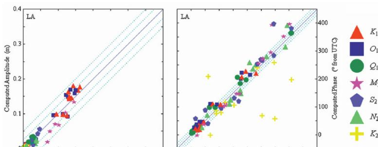
Figure 4.22 ADCIRC SL15 model performance on tidal amplitudes and phases in Louisiana
