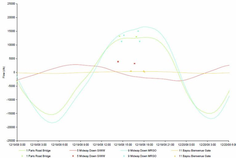
Figure 4.25 Measured and predicted flux (December 2008 ADCP survey), RMA2 study [e]
