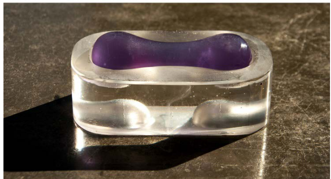
Fig.6: Type C blocks: Wall configuration. Colored (dichroic) glass has been used for the bone-shaped elements.
