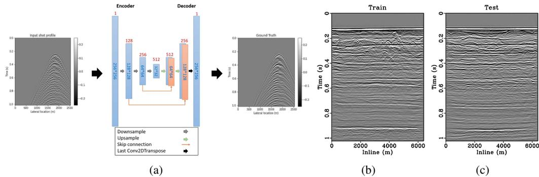
**Figure 1** U-Net architecture (a) used in this study, and two fixed-spread fully sampled subsets from the same 2D Nelson line. (b) Subset used for training. (c) Subset used for testing.
