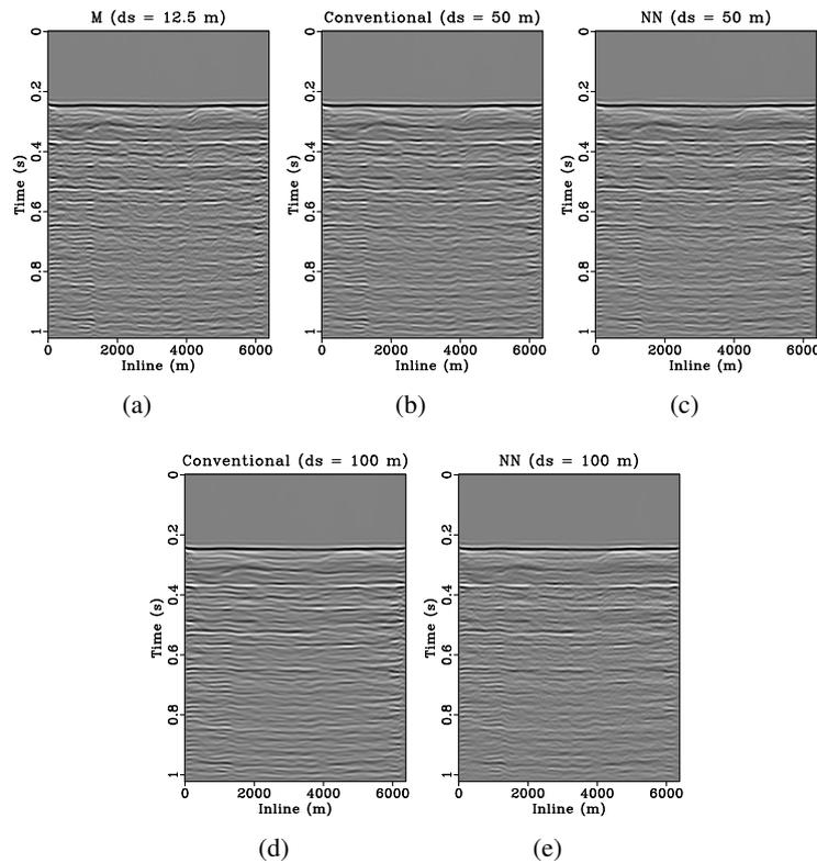
**Figure 4** Stacked section comparison for estimated multiples from (a) the original fully sampled sources (12.5 m source spacing), (b) & (c) the conventional interpolated data and the NN dealised data (50 m source spacing), and (d) & (e) the conventional interpolated data and the NN dealised data (100 m source spacing).
