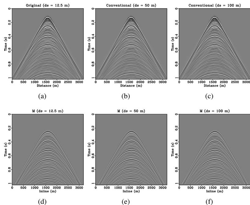
**Figure 2** Conventional source interpolation results and their corresponding estimated multiples. (a) & (d) Original shot and its multiples with 12.5 m source spacing. (b) & (e) Interpolated shot with 50 m source spacing and the estimated corresponding multiples after interpolation. (c) & (f) Interpolated shot with 100 m source spacing and the estimated corresponding multiples after interpolation.
