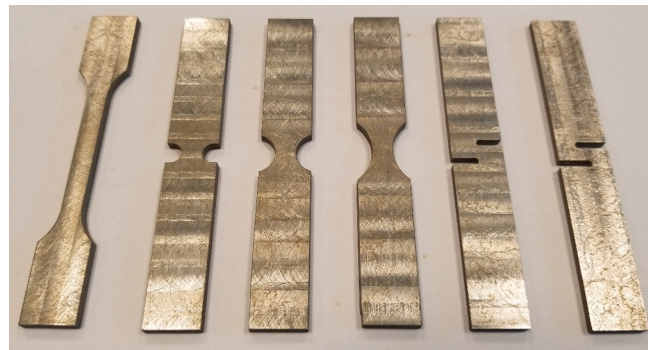
Fig. 3. Photos of milled 3D printed specimens.
