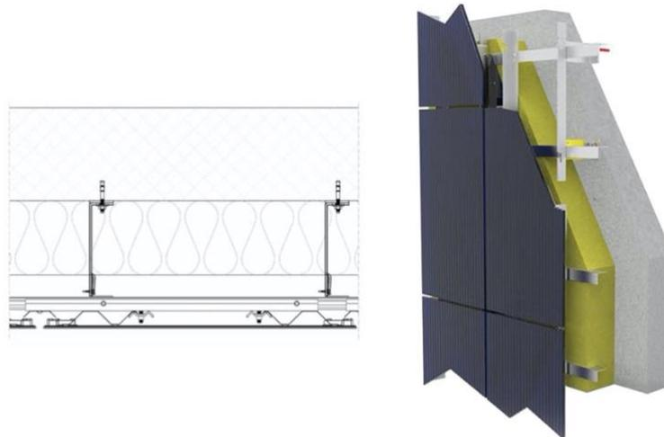
Figure 30: Example BIPV ventilated façade plan drawing (left) and façade installation diagram (right) (Avancis, 2019b).
