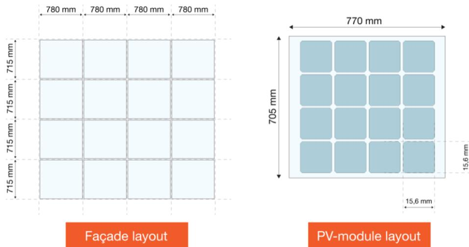
Figure 54: Façade and PV-module layouts.
