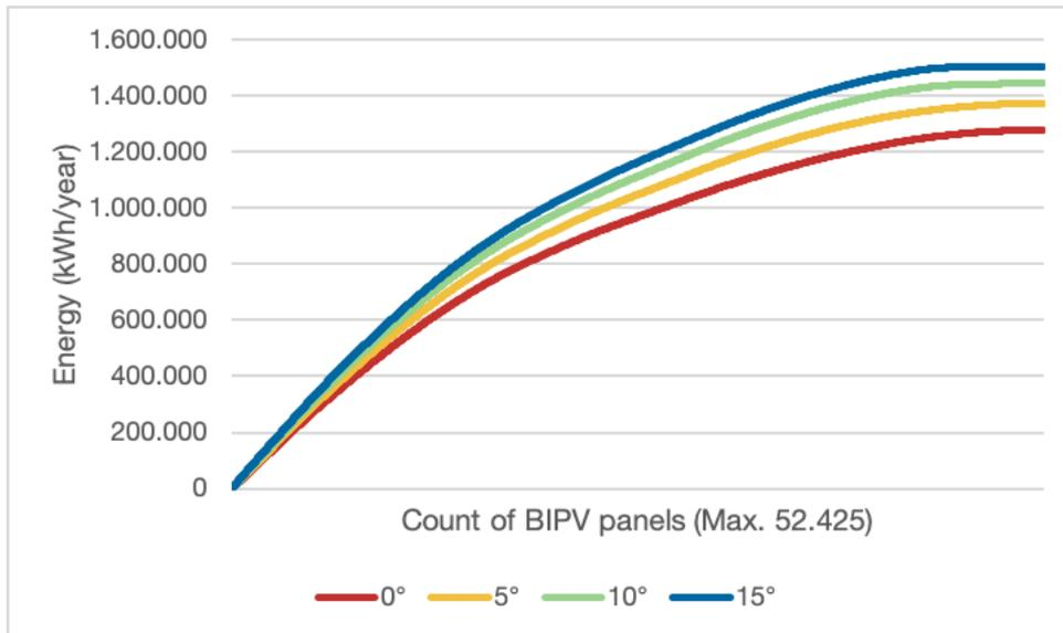
Figure 77: Scenario-0, energy generation with each additional BIPV-module.
