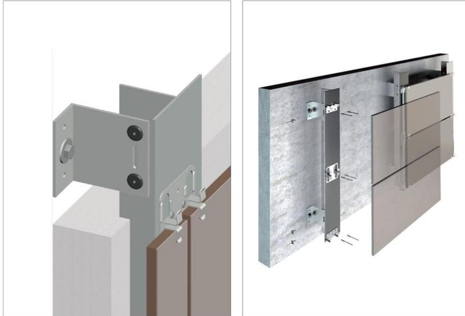
Figure 28: Visible anchoring system (Marazzi Engineering, 2019).
