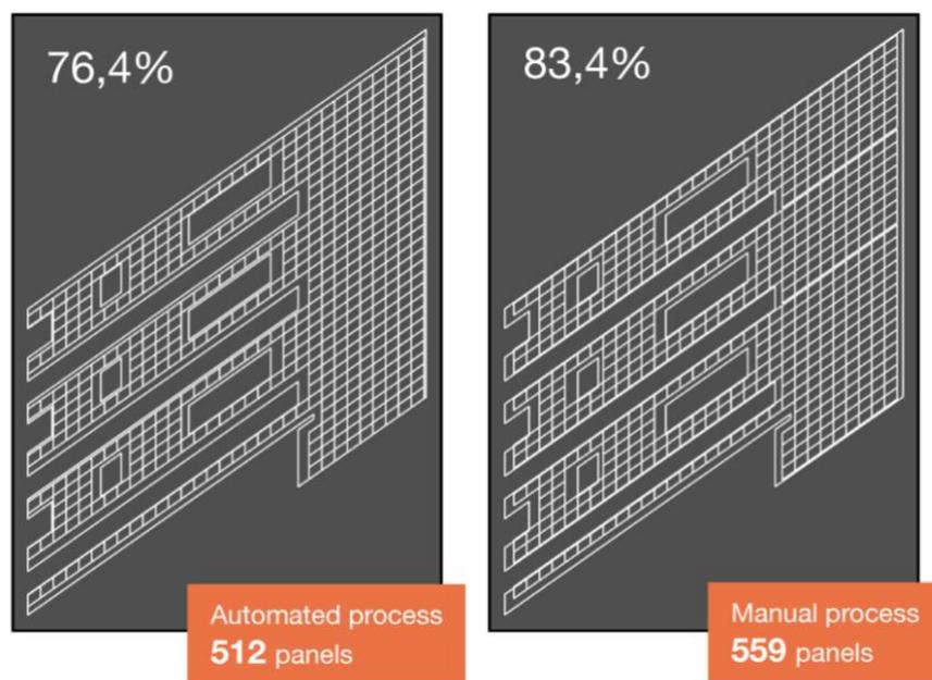
Figure 70: Comparison of the manual and the automated panelling.
