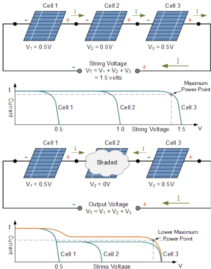
Figure 13: Shading of a single cell in a string causes a significant reduction in the MPP (Alternative Energy Tutorials, 2018).
