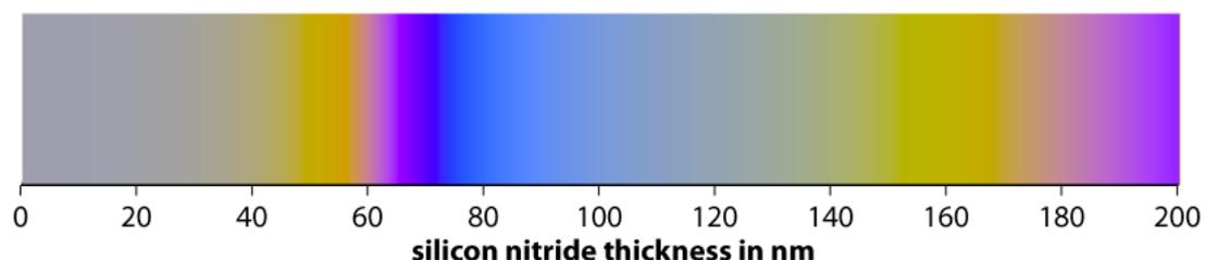
Figure 20: Colour of silicon nitride films as a result of film thickness under fluorescent light (Honsberg & Bowden, 2019a).
