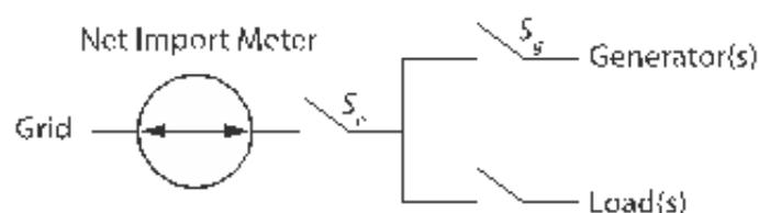
Figure 10: Net-metering diagram 1 (GSES, 2013).
