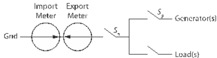
Figure 11: Net-metering diagram 2 (GSES, 2013).
