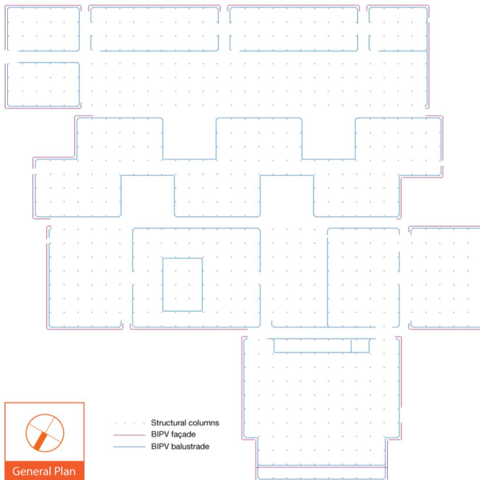
Figure 52: The horizontal alignment of the standardised panels on the façade and the balustrades all around the building.
