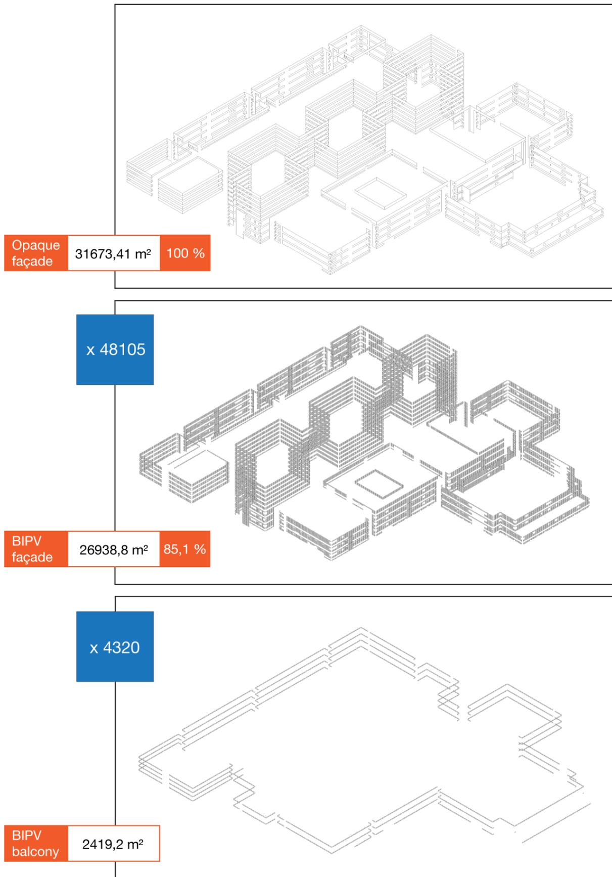
Figure 53: Panel distribution as a result of pre-allocation.
