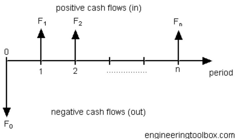
Figure 7: Example cash flow diagram (Engineering ToolBox, 2009).
