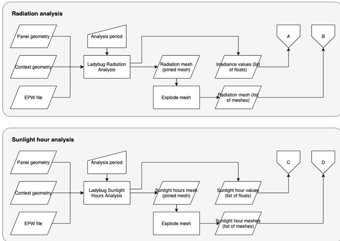
Figure 65: Inputs and outputs of the radiation and sunlight hours analysis.
