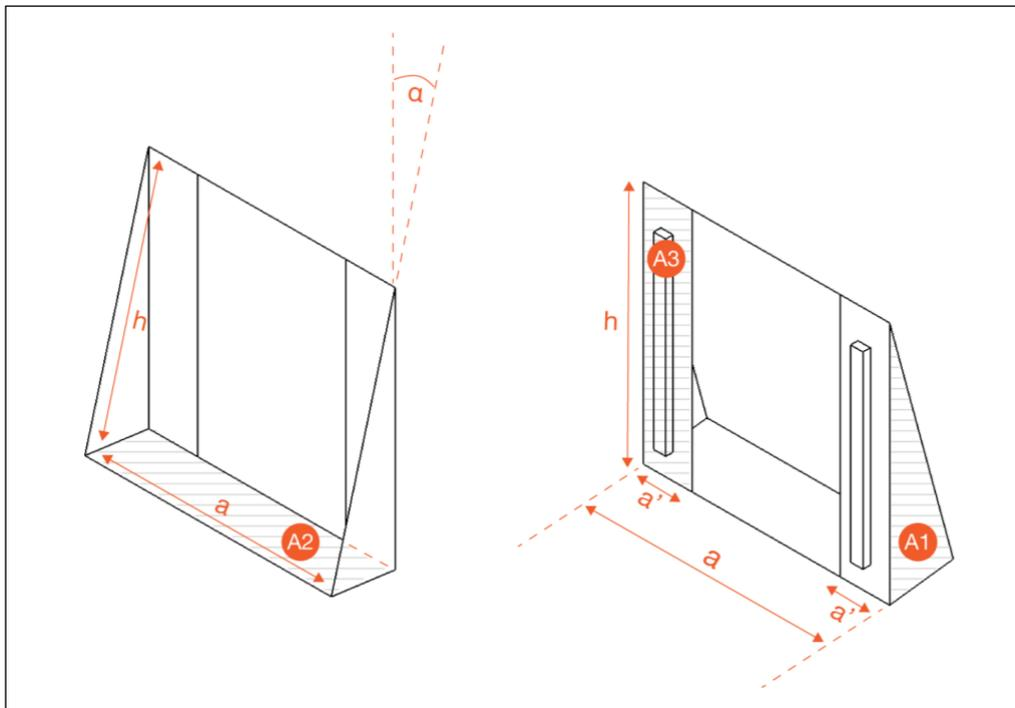
Figure 64: The geometry of the panels for cost calculation.
