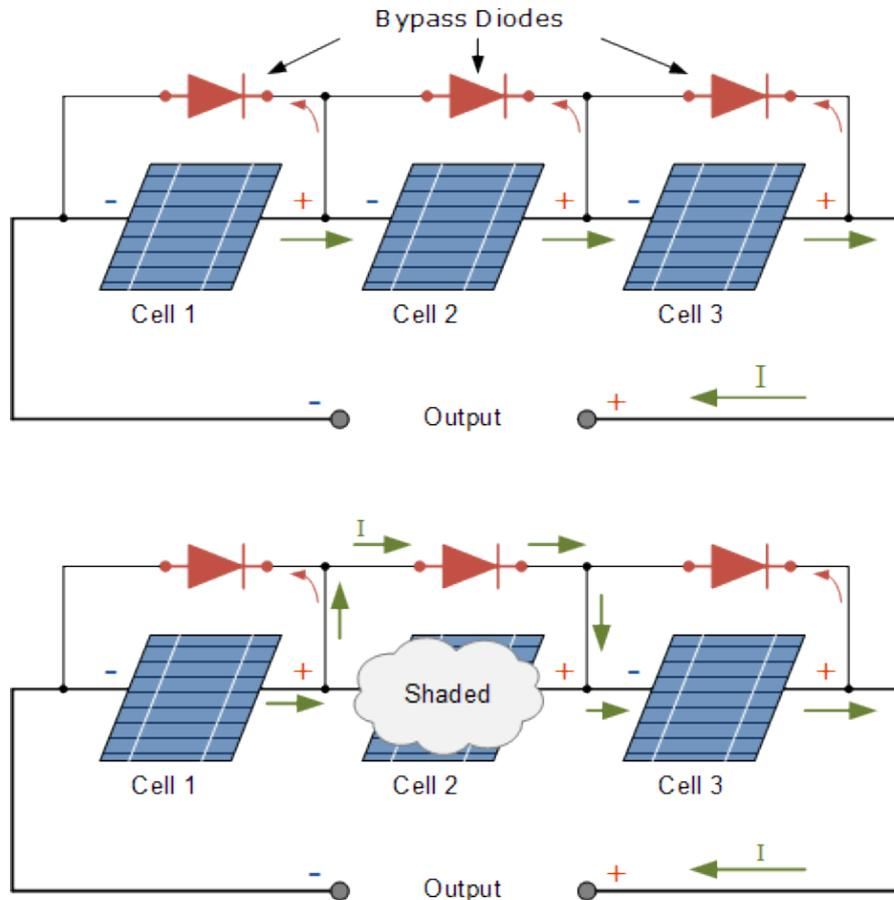
Figure 15: Bypass diodes prevent hotspot heating by preventing the current run through the shaded PV-cell (Alternative Energy Tutorials, 2018).
