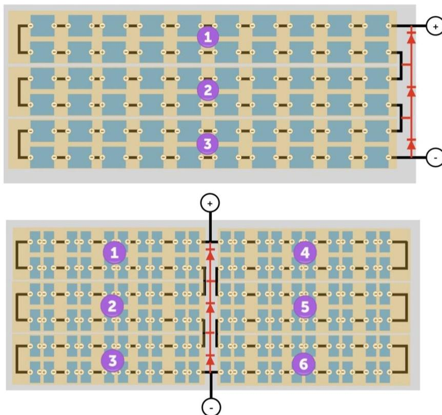
Figure 16: Comparison of 3-string full cell panel and 6-string half-cut cell panel, bypass diodes shown in red (Brakels, 2018).
