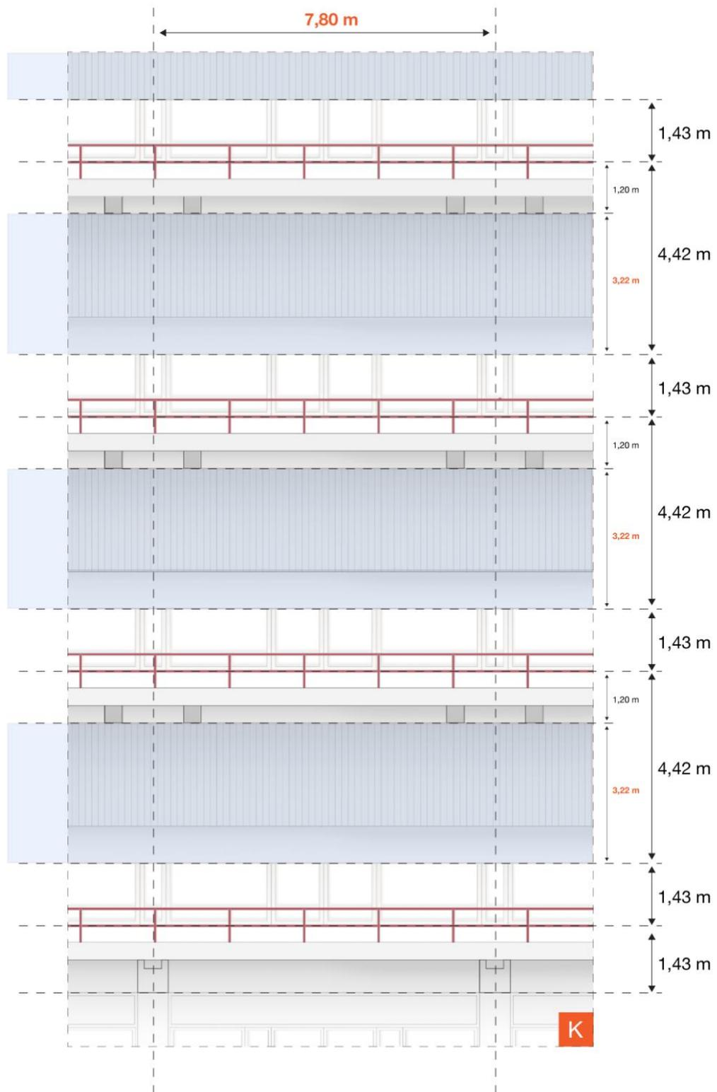
Figure 51: Partial elevation of the block K with its dimensions.
