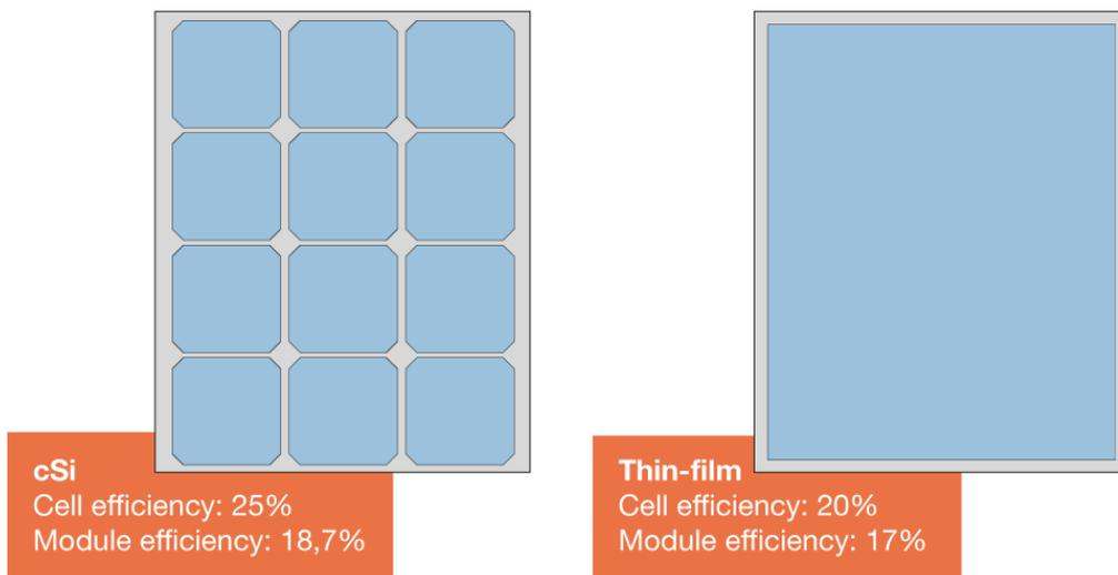
Figure 88: Possible PV technologies for the BIPV panels.
