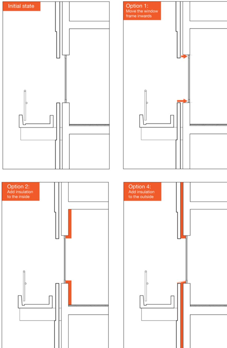
Figure 47: Initial state of the façade and the options for thermal improvement.
