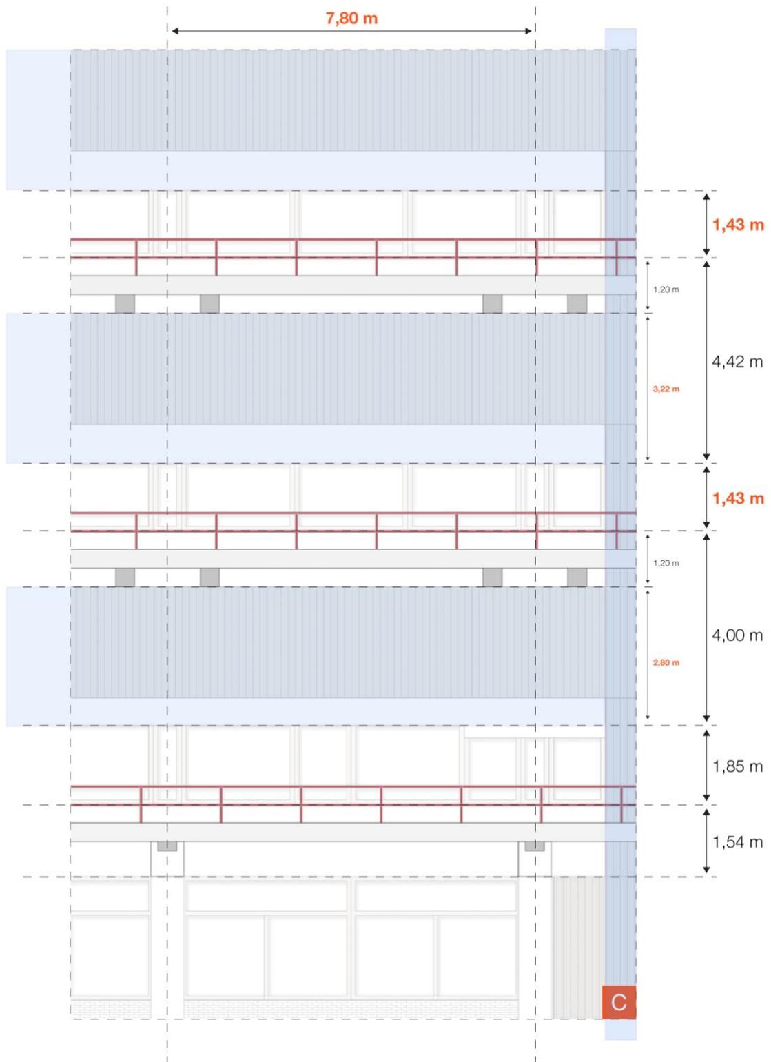
Figure 49: Partial elevation of block C with its dimensions.
