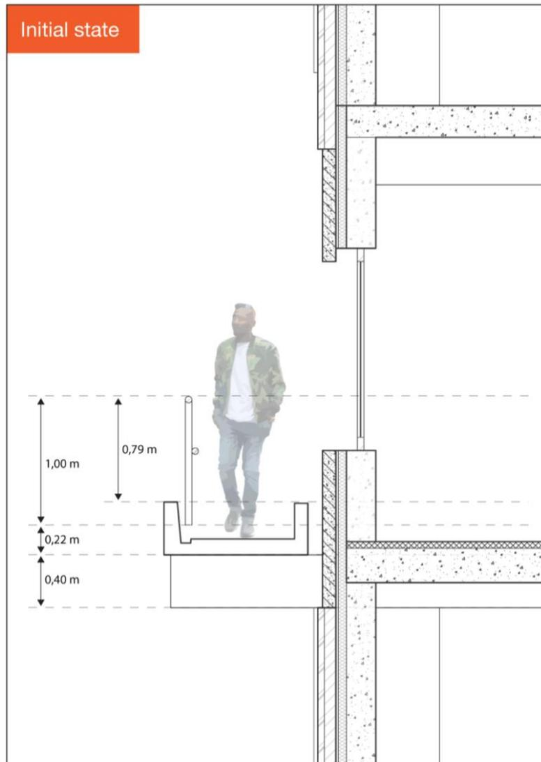
Figure 61: Initial state of the balconies.
