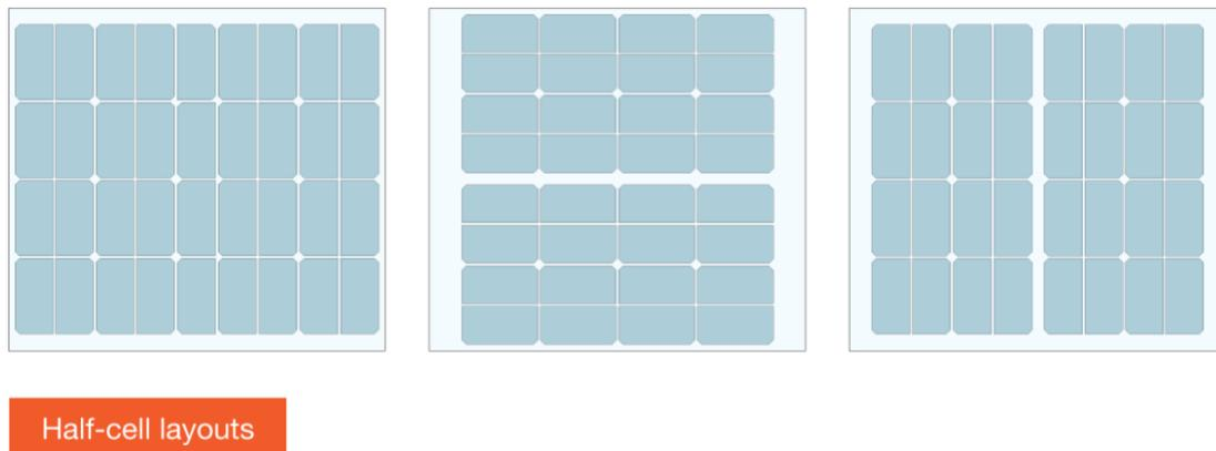
Figure 55: Module layouts with half-cut cells
