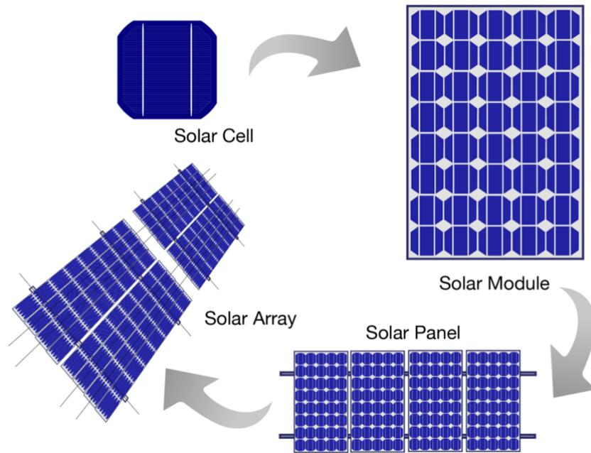
Figure 9: The relation between PV-cell -module and -array.
