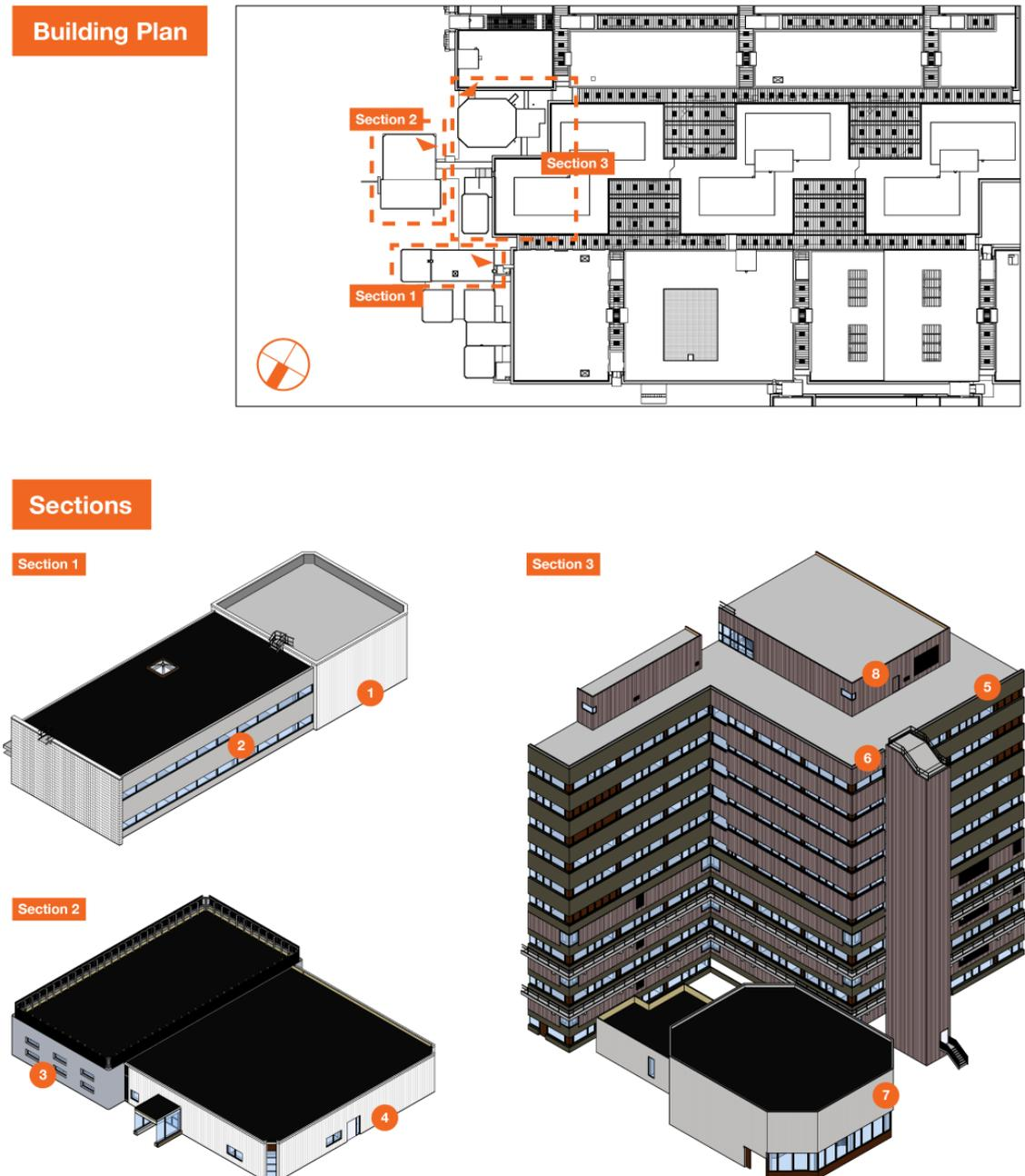
Figure 34: Different façade types (1 to 8) and their position in the building.
