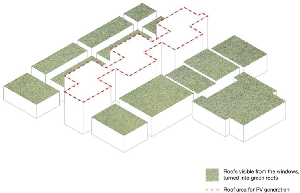
*Figure 41: If the roof visible from the bed towers are turned into green roofs, very small area is left for energy generation.*
