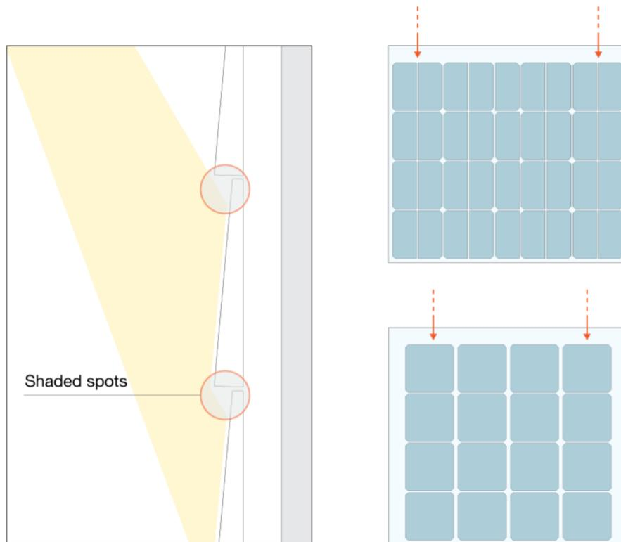
Figure 58: In the tilted modules, the cells can be shifted downwards to avoid the shading caused by the module above.
