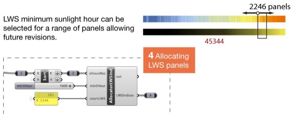
Figure 85: Allocating the LWS panels according to their minimum sunlight hour requirement.
