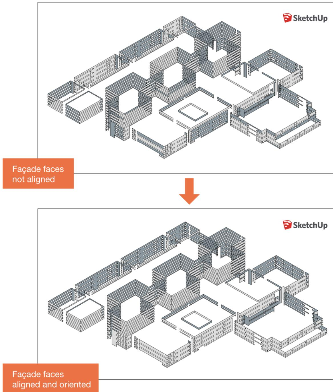
Figure 68: The faces of the façade geometry should be aligned and oriented correctly before being put to process.
