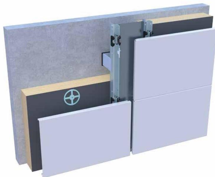
Figure 31: Façade composition with the click system (Kalzip, 2019)
