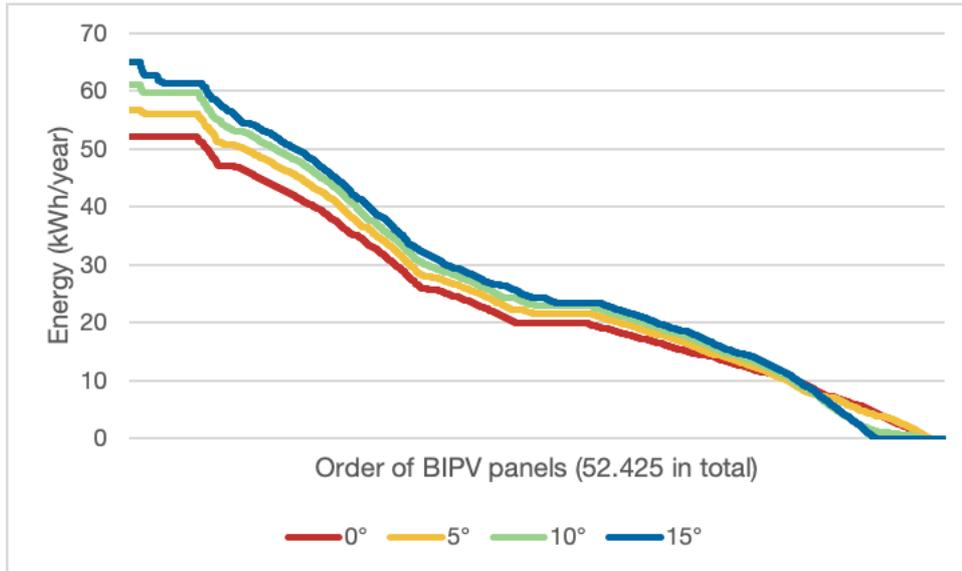
Figure 76: Scenario-0, energy generation of each BIPV-module, descending sort.
