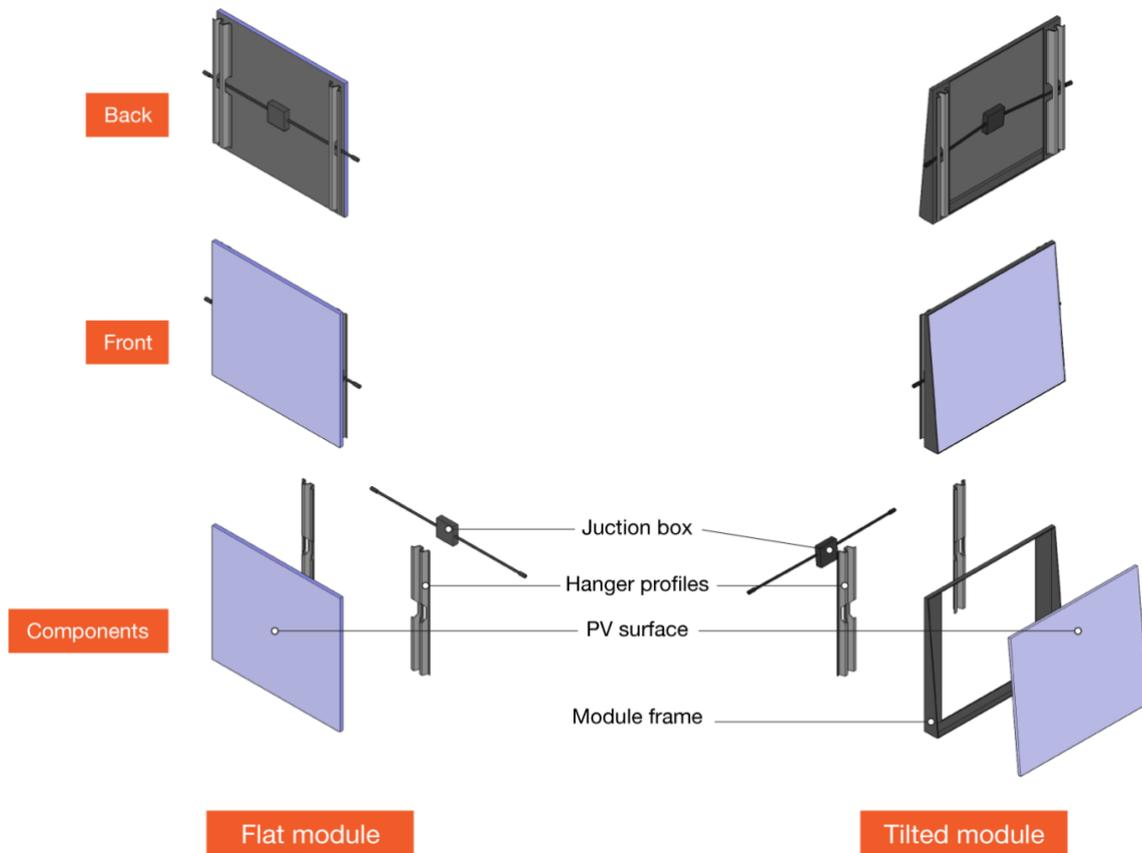
Figure 60: The front and back view of the modules, with their components.
