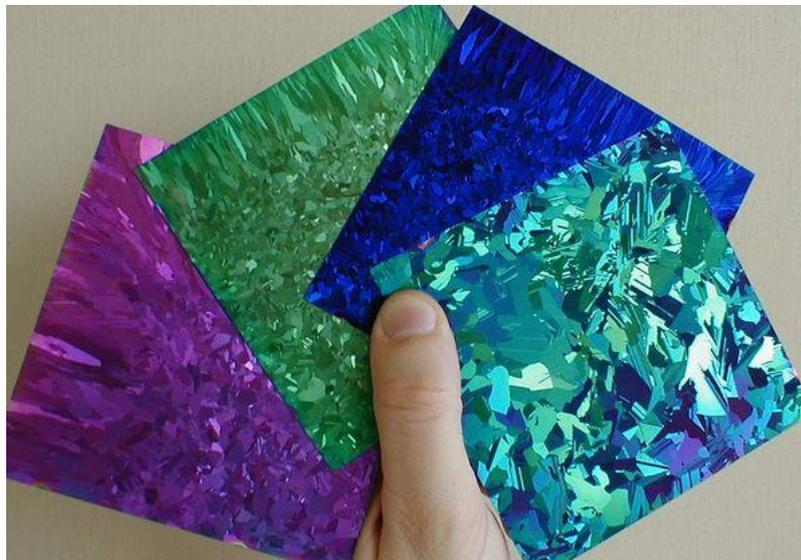
Figure 19: Multi-crystalline wafers coated with silicon nitride (Honsberg & Bowden, 2019a).
