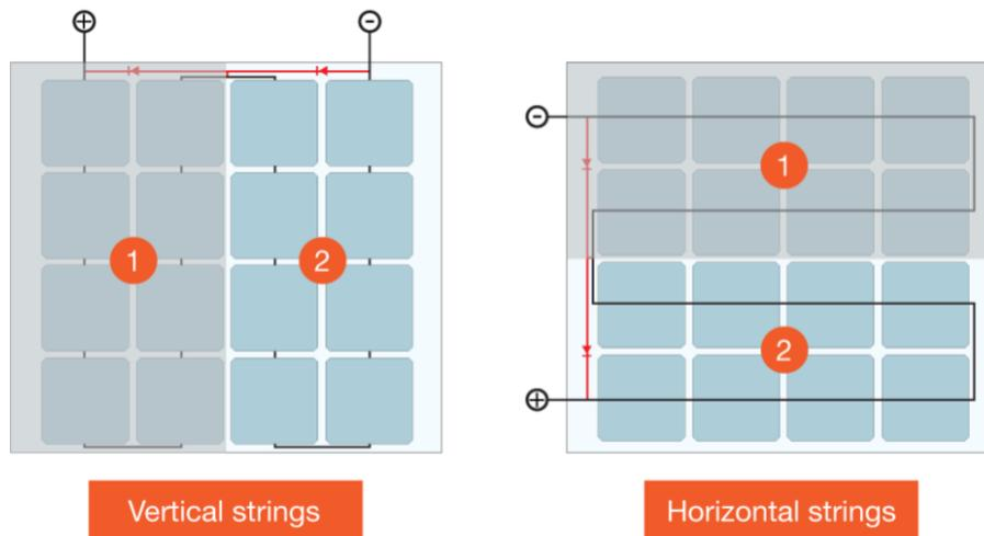
Figure 56: The string directions in the modules can be determined to minimise the effect of shading.
