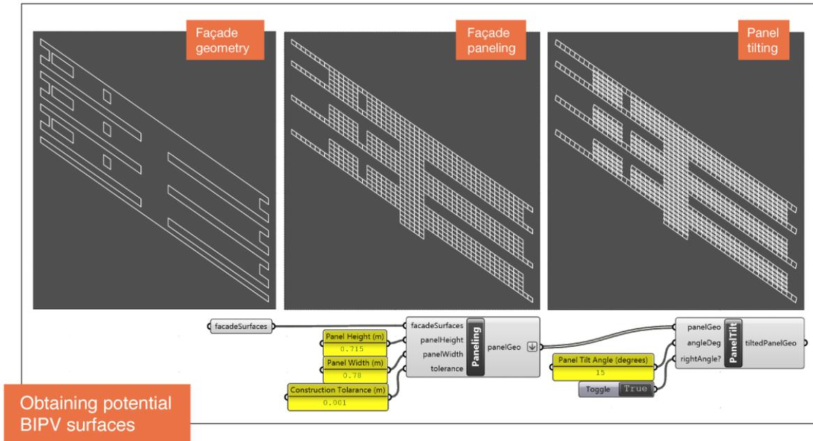
Figure 66: Example grasshopper definition for creating the panel geometries for solar analyses.
