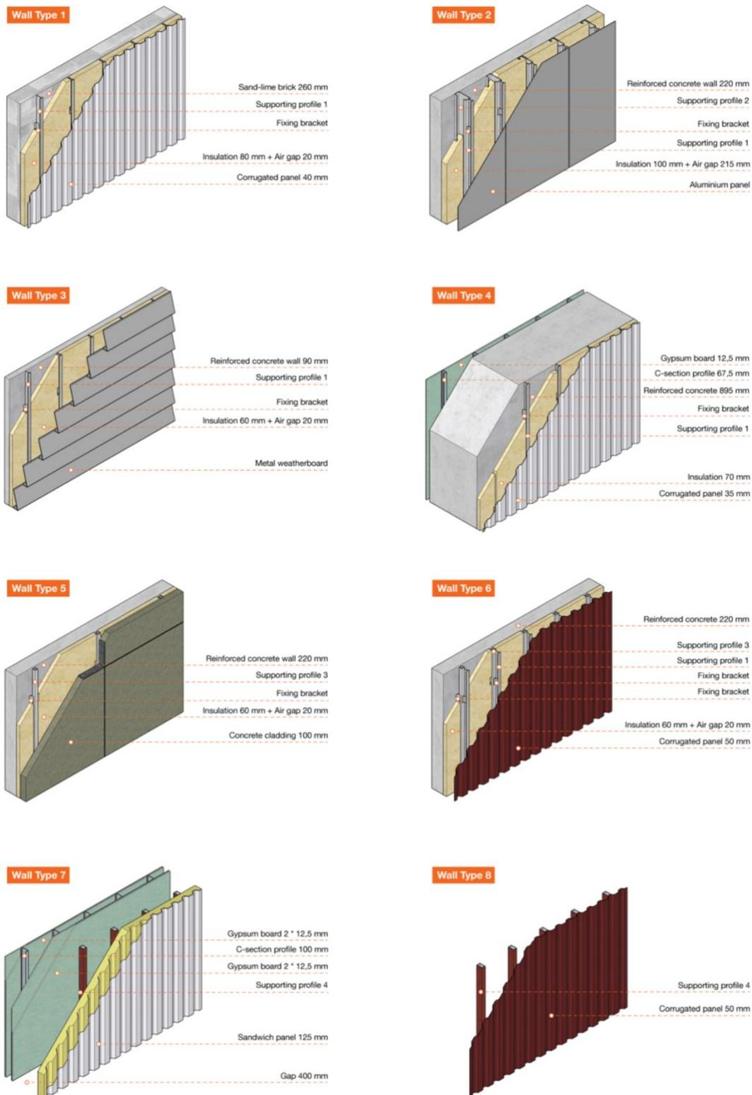
Figure 35: Components of the façades. Materials and layer thicknesses were taken from the BIM-model, but the substructures were interpreted.
