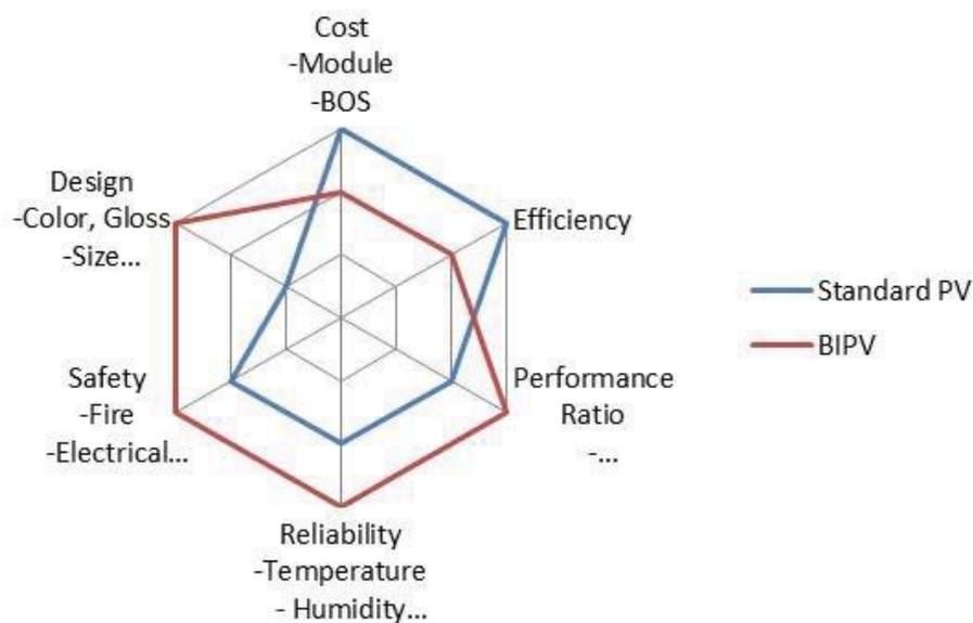
Figure 18: Requirement comparison for standard PV and BIPV (Palm et al., 2018)
