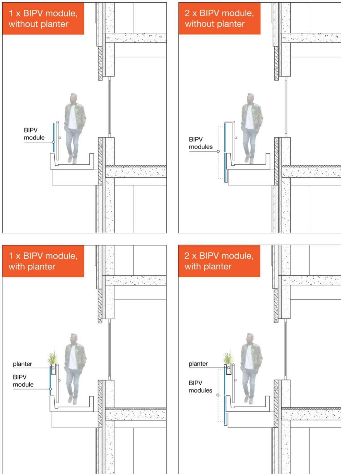
Figure 62: Different options for using the balustrades as BIPV surfaces.
