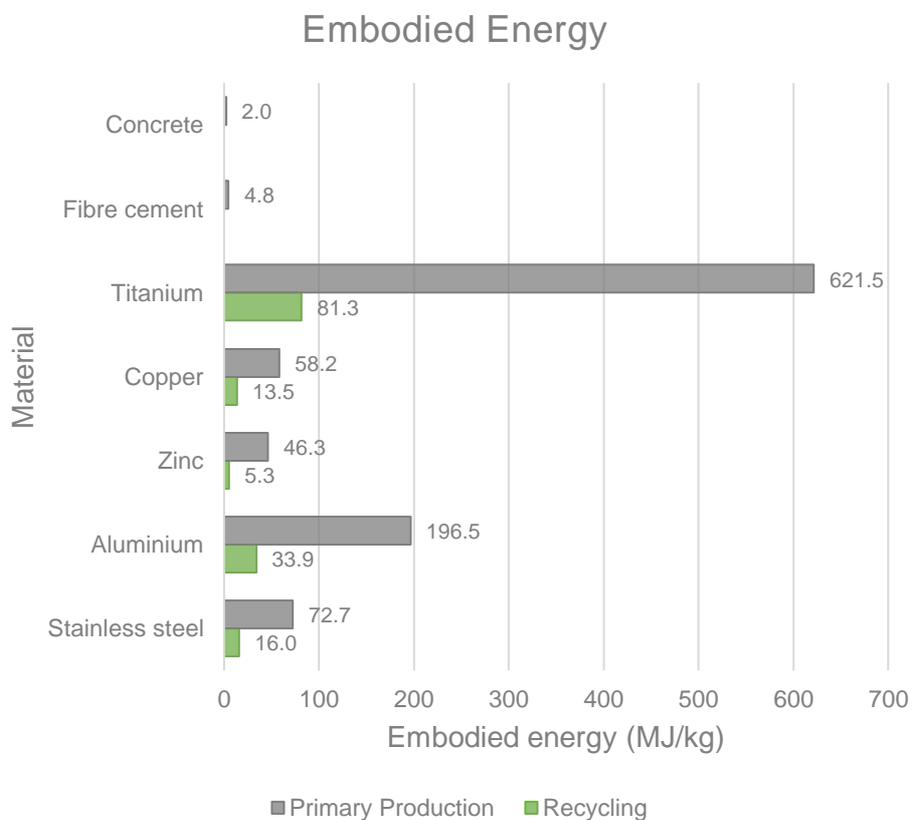
Figure 44: Material options, embodied energy comparison.
