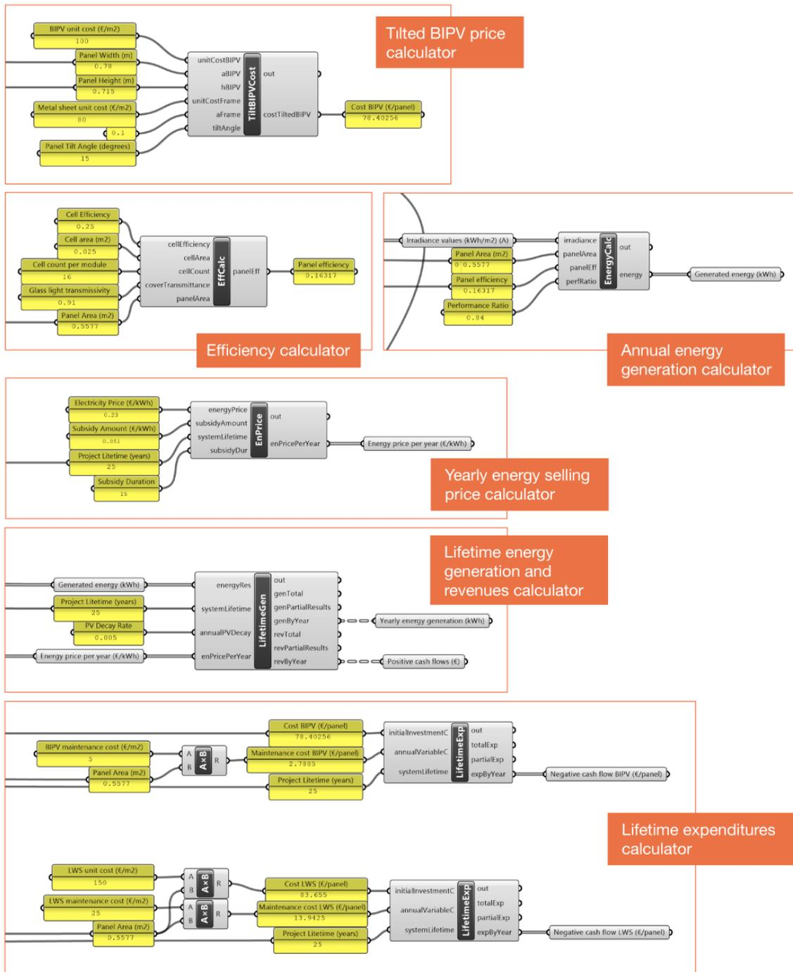
Figure 72: The tools used for calculating the cash flows.
