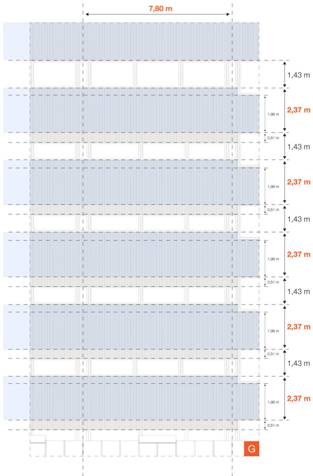
Figure 50: Partial elevation of the block G with its dimensions.
