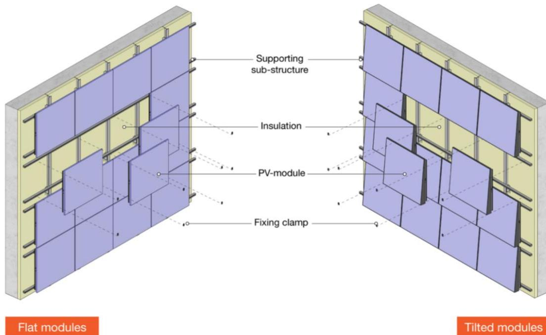
*Figure 59: The façade system with flat and tilted panels.*
