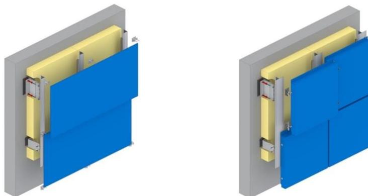
Figure 29: Examples of concealed anchoring system (IPEX, 2020).
