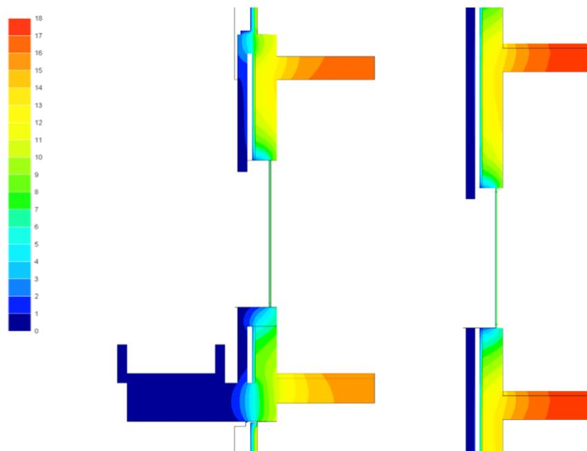
Figure 36: Steady-state thermal simulation results of AMC low-rise (left) and high-rise (right) (DGMR Bouw, 2016).
