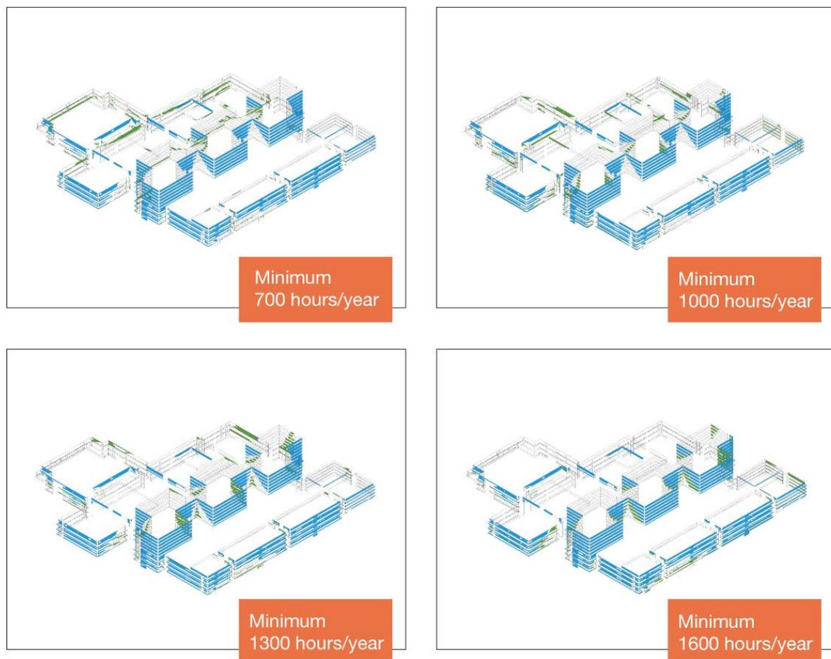
Figure 86: Computationally allocated BIPV and LWS panels with different minimum sunlight hours, affecting the positioning of the LWS panels.
