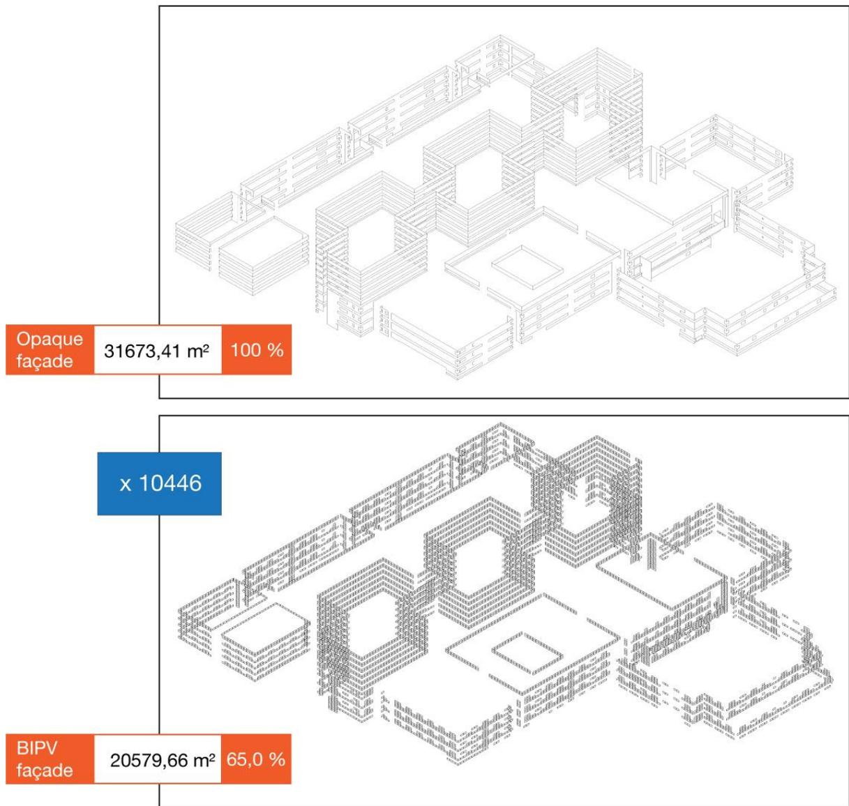
Figure 42: Distribution of standard PV-module son the opaque walls of AMC.
