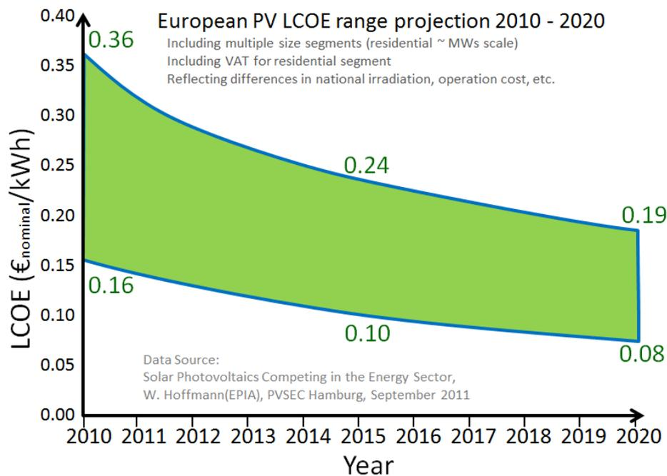
Figure 17: Graph showing the drop in the PV LCOE in Europe.
