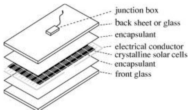
Figure 22: Layers of a generic c-Si PV-module (Schulze et al., 2012).
