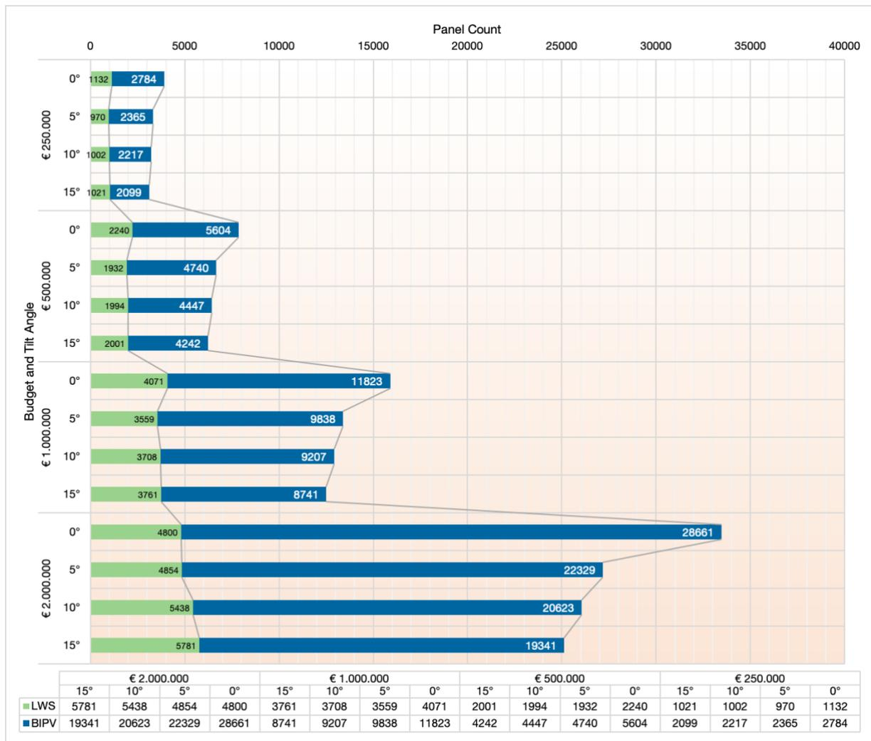
Figure 83: The optimum panel counts to pay off the investment costs with most LWS panels with different budgets and tilt angles.
