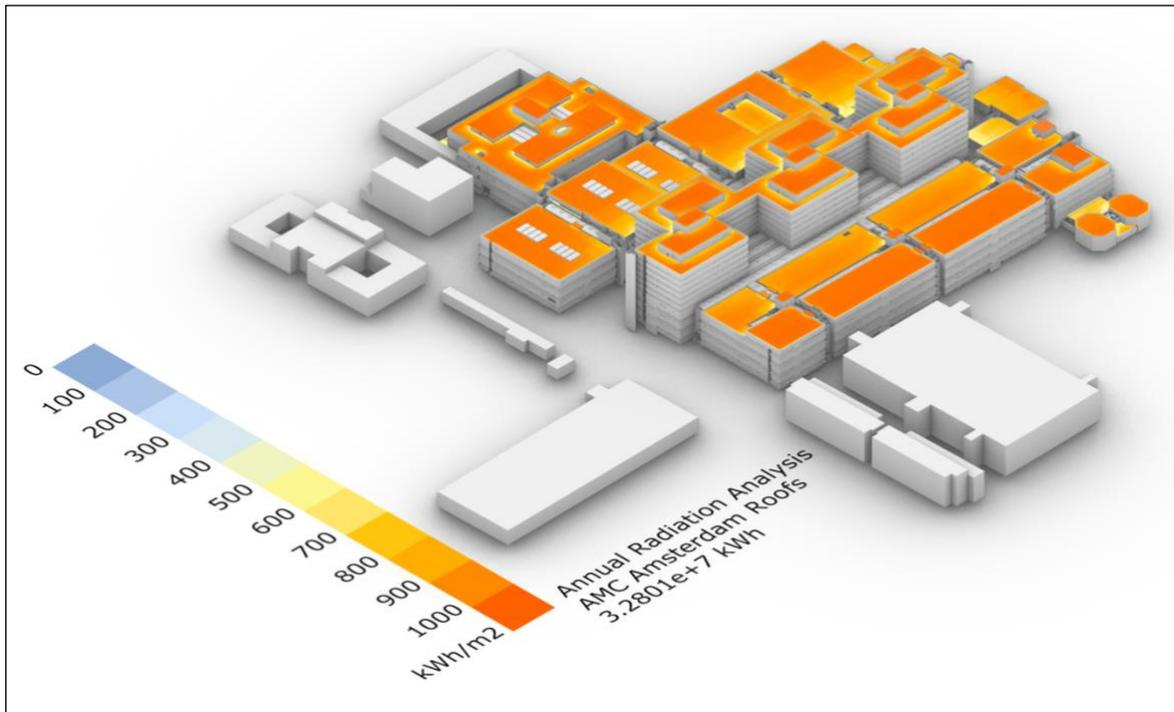
Figure 40: Roof insolation analysis result (view from the North).
