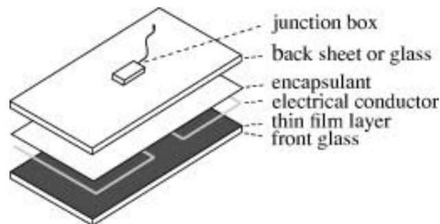
Figure 23: Layers of a generic thin-film PV-module (Schulze et al., 2012).
