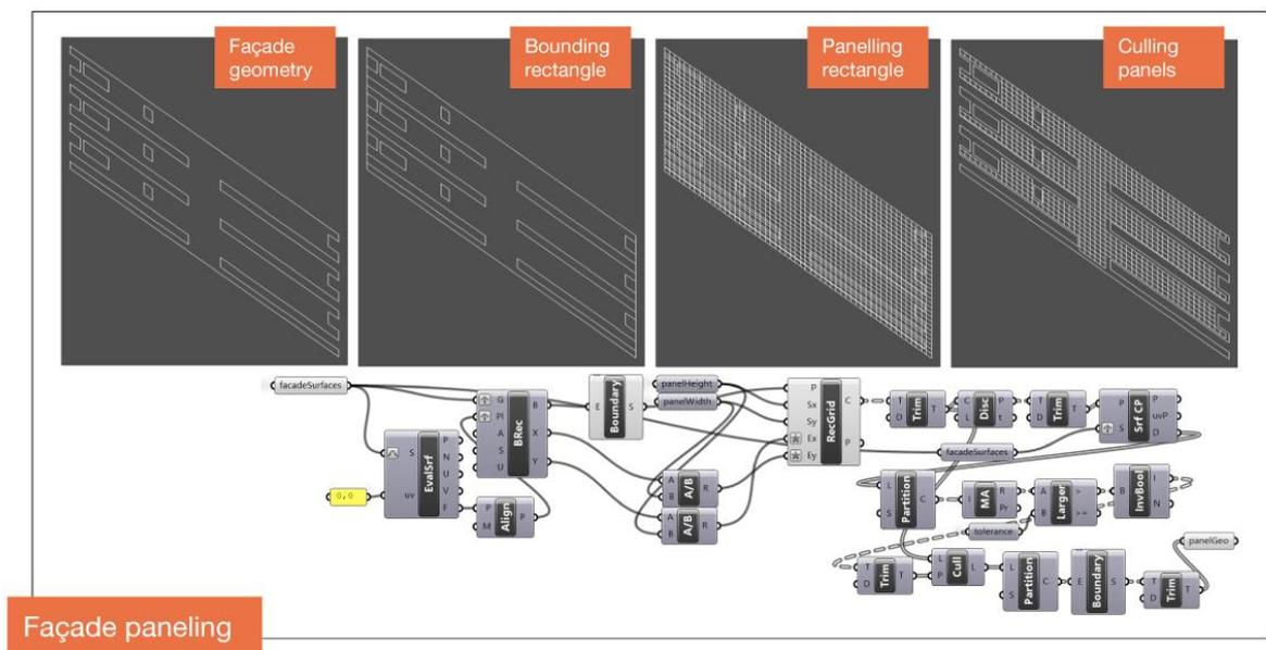
Figure 67: Content of the panelling tool.
