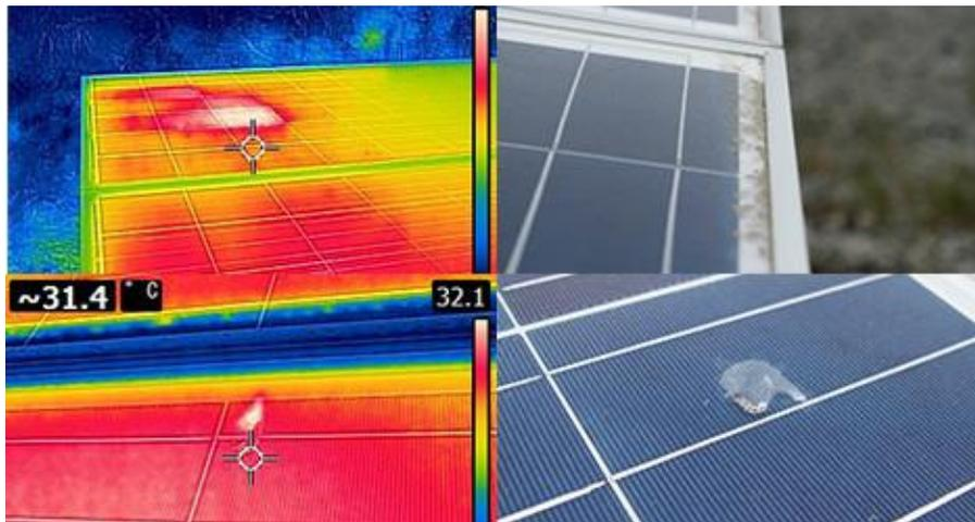
Figure 14: The damaging effects of hotspot heating (Skyrobot Inc., n.d.).
