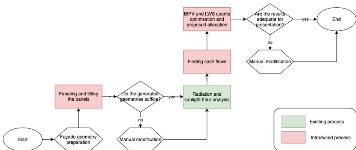
Figure 63: Flowchart of the proposed methodology for computational design and optimisation.
