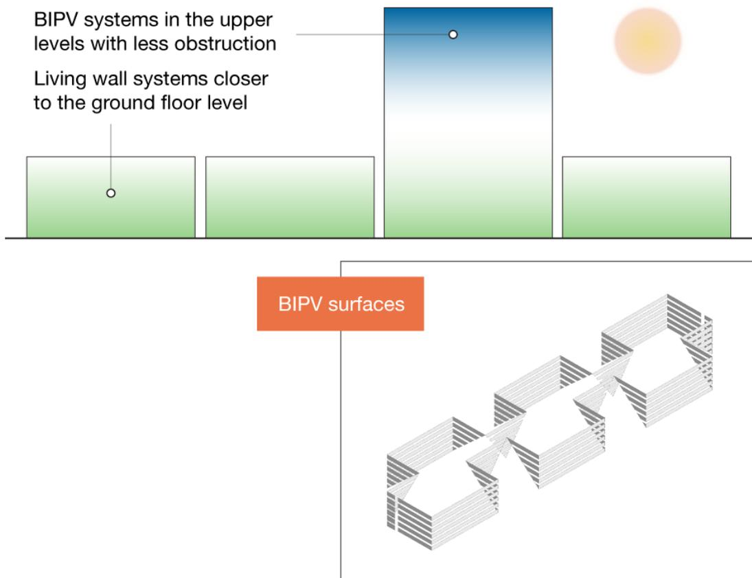
*Figure 87: An example façade design decision and the façade surface to be covered with BIPV panels.*
