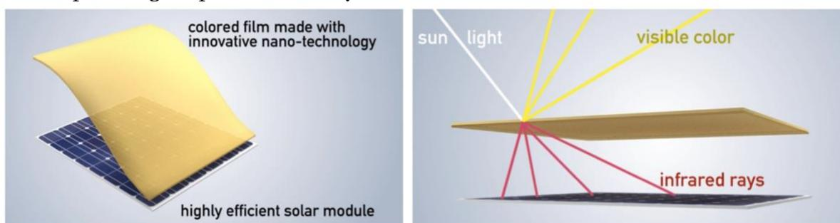
Figure 21: Selective film applied on the c-Si PV-module (Solaxess, n.d.).
