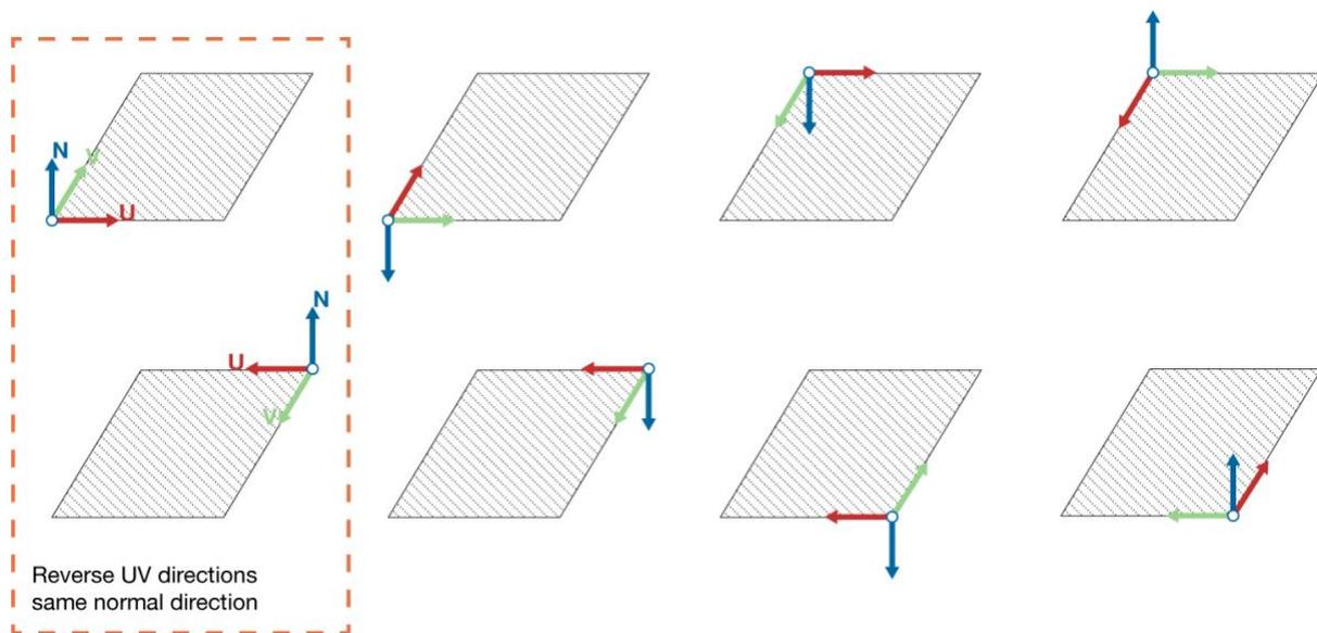
Figure 69: Faces may have reversed U and V direction even when facing the same direction.
