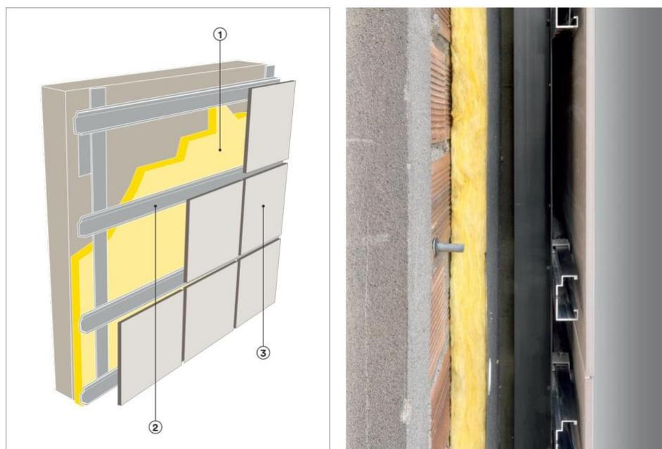
Figure 27: Ventilated façade layers (left): insulation (1), supporting substructure (2), façade cover (3) and a photograph of a ventilated façade system (right) (Marazzi Engineering, 2019).
