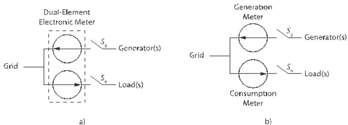
Figure 12: Gross metering diagram (GSES, 2013).
