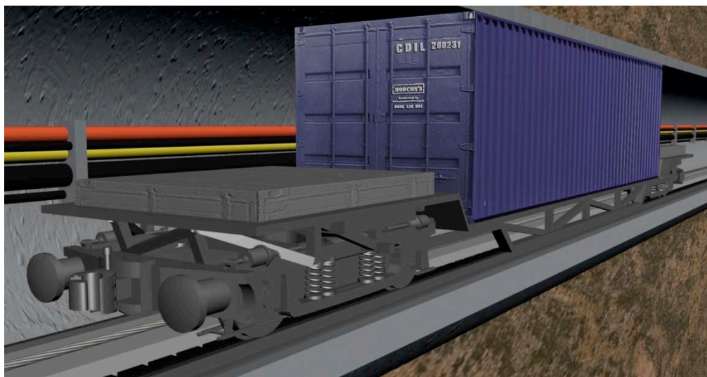
FIGURE 1: THE UCM ® (Denys NV) Underground Container Mover WITH TRANSPORT CHAINS IN A LOOP, LOW BED TRAILERS AND ELECTRIC MOTORS.
