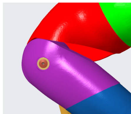
Figure 6: Figure showing degrees of freedom, and the cutout portion/clearance for left knee joint
