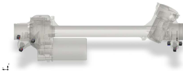
Fig. 12 Electric power steering setup with a 6-DoF virtual point on the left and right sides
