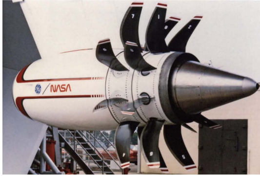
Figure 1.1: Concept counter-rotating turboprop engine on test stand. [1]
