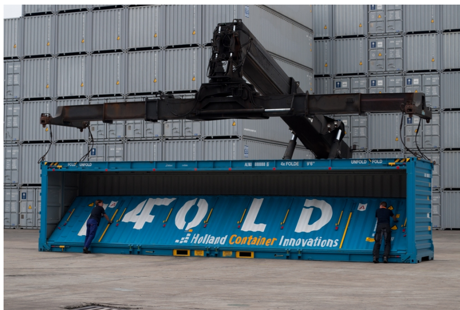
Figure 26 Demonstration of a 40-foot folding container. Note that it requires 3 people and a crane to operate. Source: (Holland Container Innovations, 2018)
