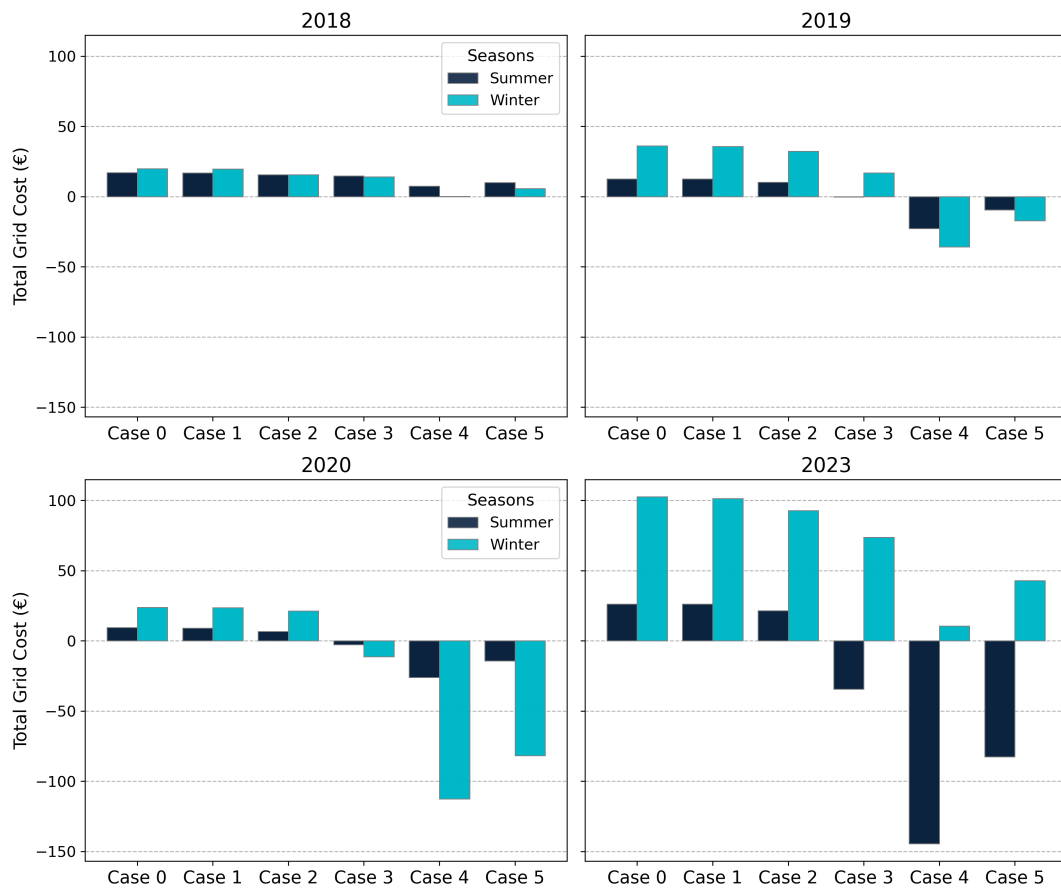
Figure 6.2.2: Total grid sum for each case, year and season. Grid cost consists of both cost of imported energy, as revenue from aFRR participation and exported energy.
