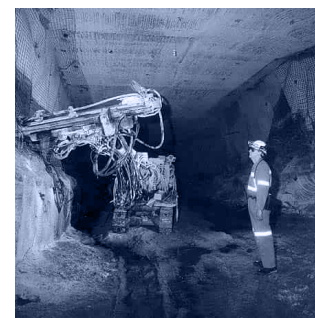
Fig. 18 - Paul Deakin, Rock Fig. 19 - Joe Raedle, open- bolting in the Boulby pit copper mine in New potash mine, Mexico.
