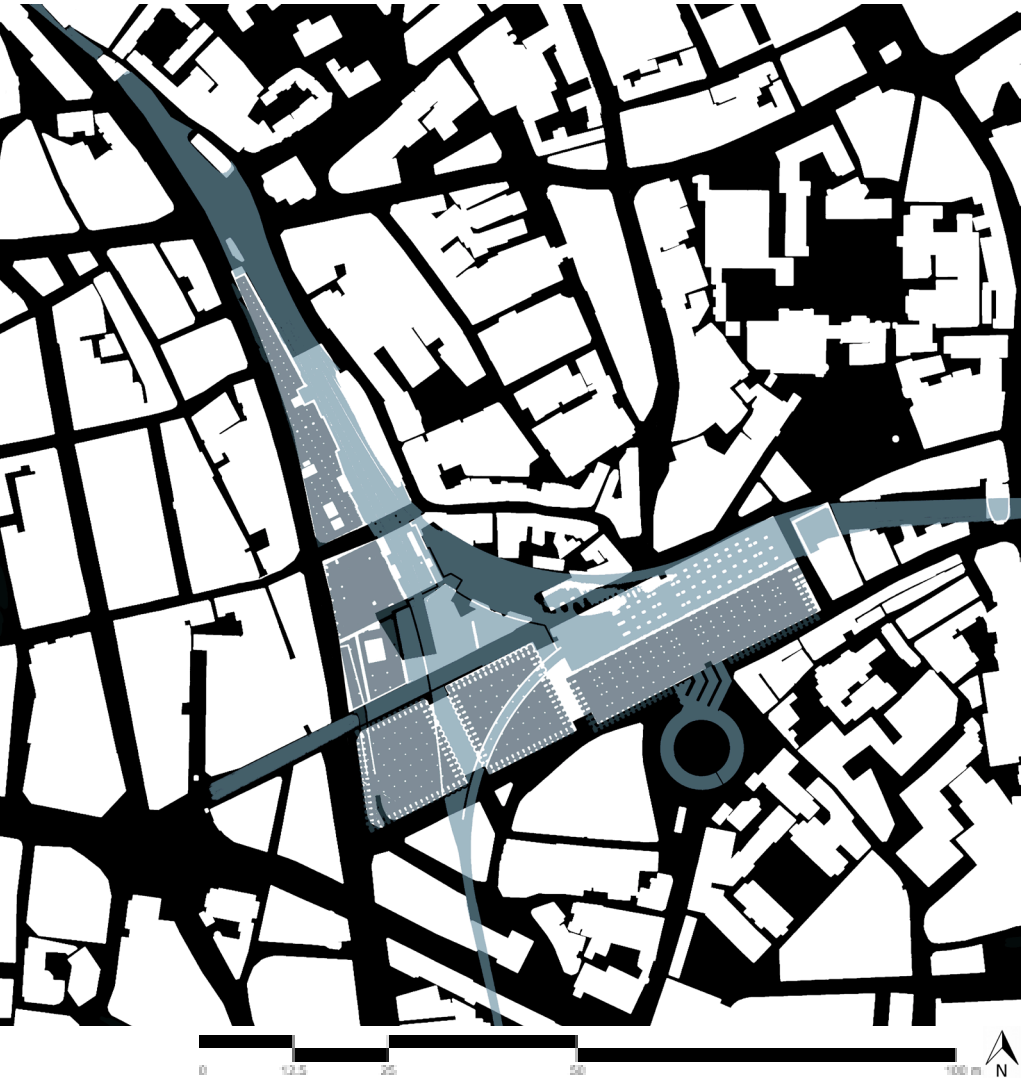
Underground space around Farringdon station area: basements, railway cuttings, and connections between buildings under the street.
