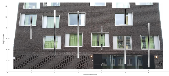
(c) Height estimation of windows overlaid on the facade of the building itself. Note that the height axis does not align with the actual height of the building, it is merely included for illustration purposes
