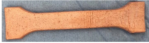
(a) Dog-bone before tensile testing
