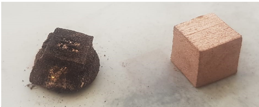
(b) Melted cube and sintered hollow cube, sintered at 1095\text{ }^\circ\text{C}
