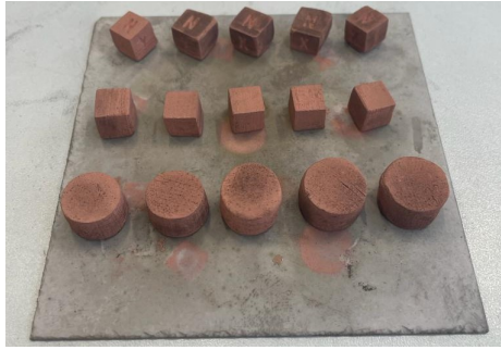
Figure 71: S16 sample set at 1075 °C in vacuum for 10 hours
