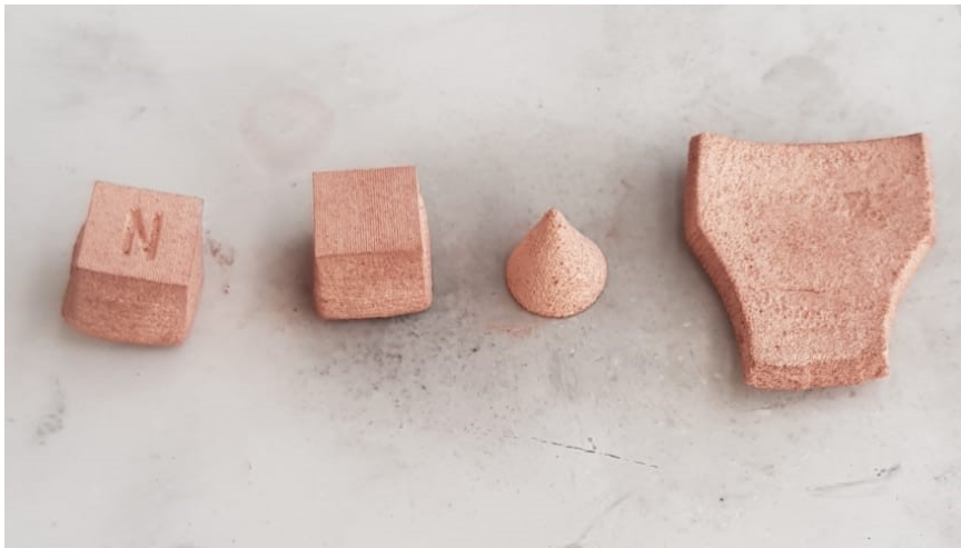
(b) Sintered samples at 1093 °C, with a distorted dog-bone piece
