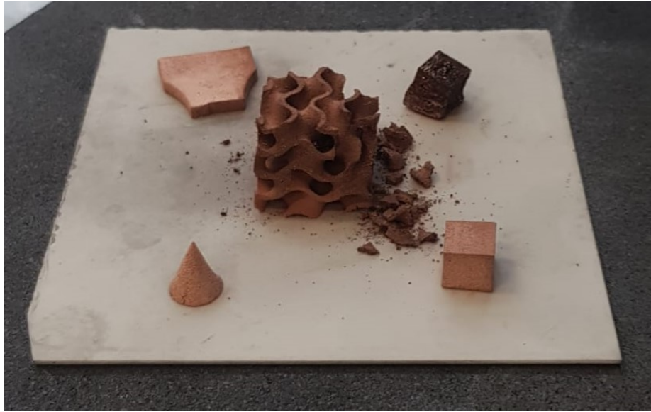
Figure 54: Sintered broken off gyroid
