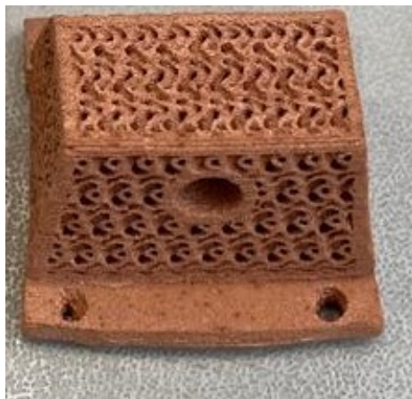
Figure 52: Distorted heat exchanger
