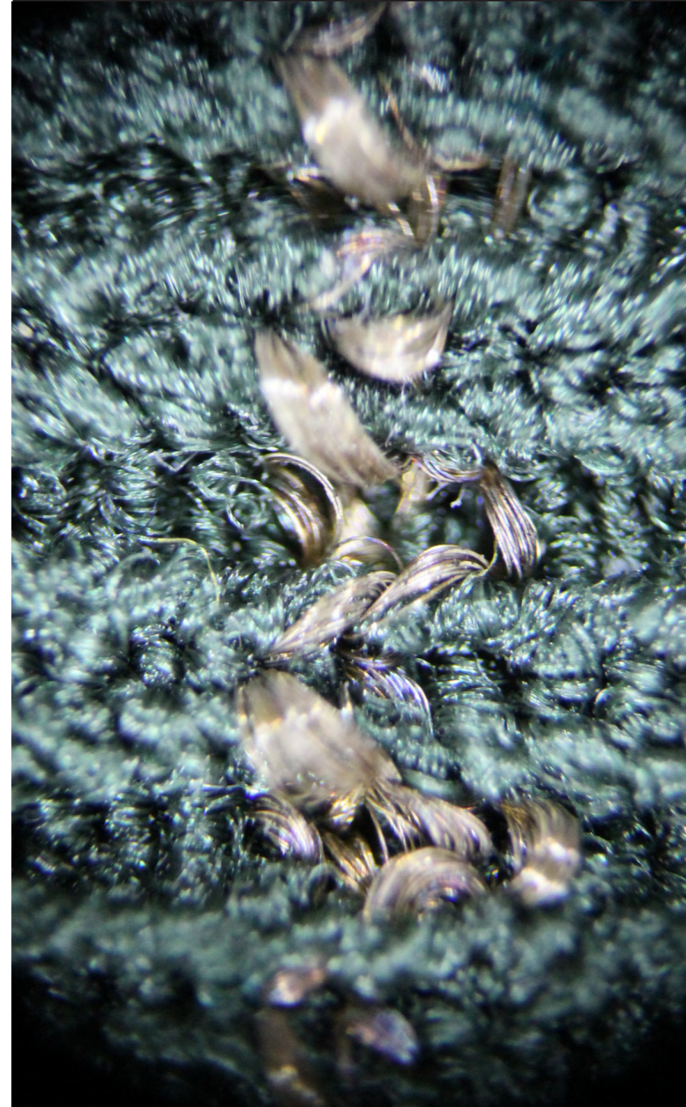
Figure 17. A knitted sensor; the conductive yarn is integrated as a three-dimensional pattern in the knitted structure
