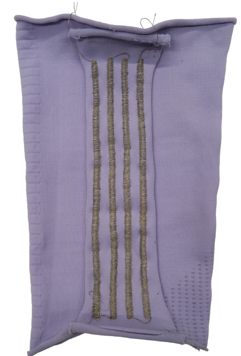
Figure 47. Four yarn rows are stitched onto a separate piece of fabric and stitched onto the sleeve
