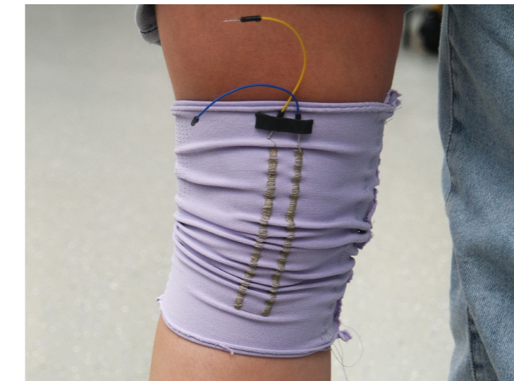
Figure 49. The sleeve has slipped causing the sensor to fold
