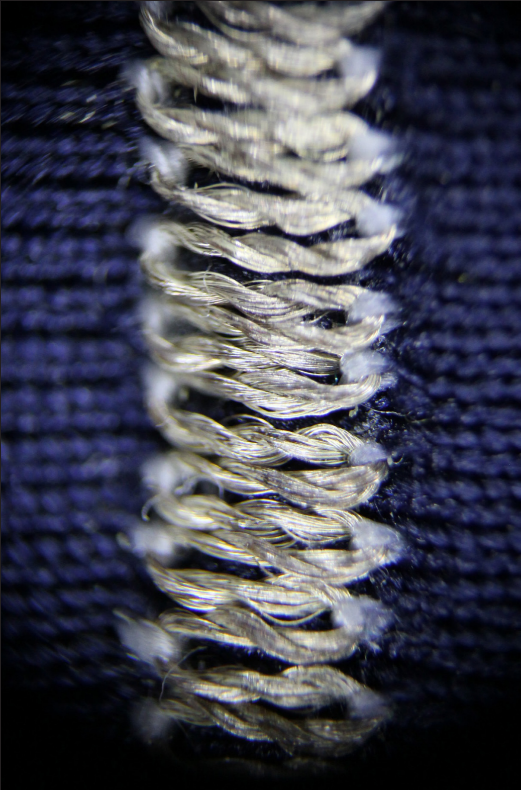
Figure 18. A stitched sensor; the yarn is stitched as a zigzag structure onto the base fabric
