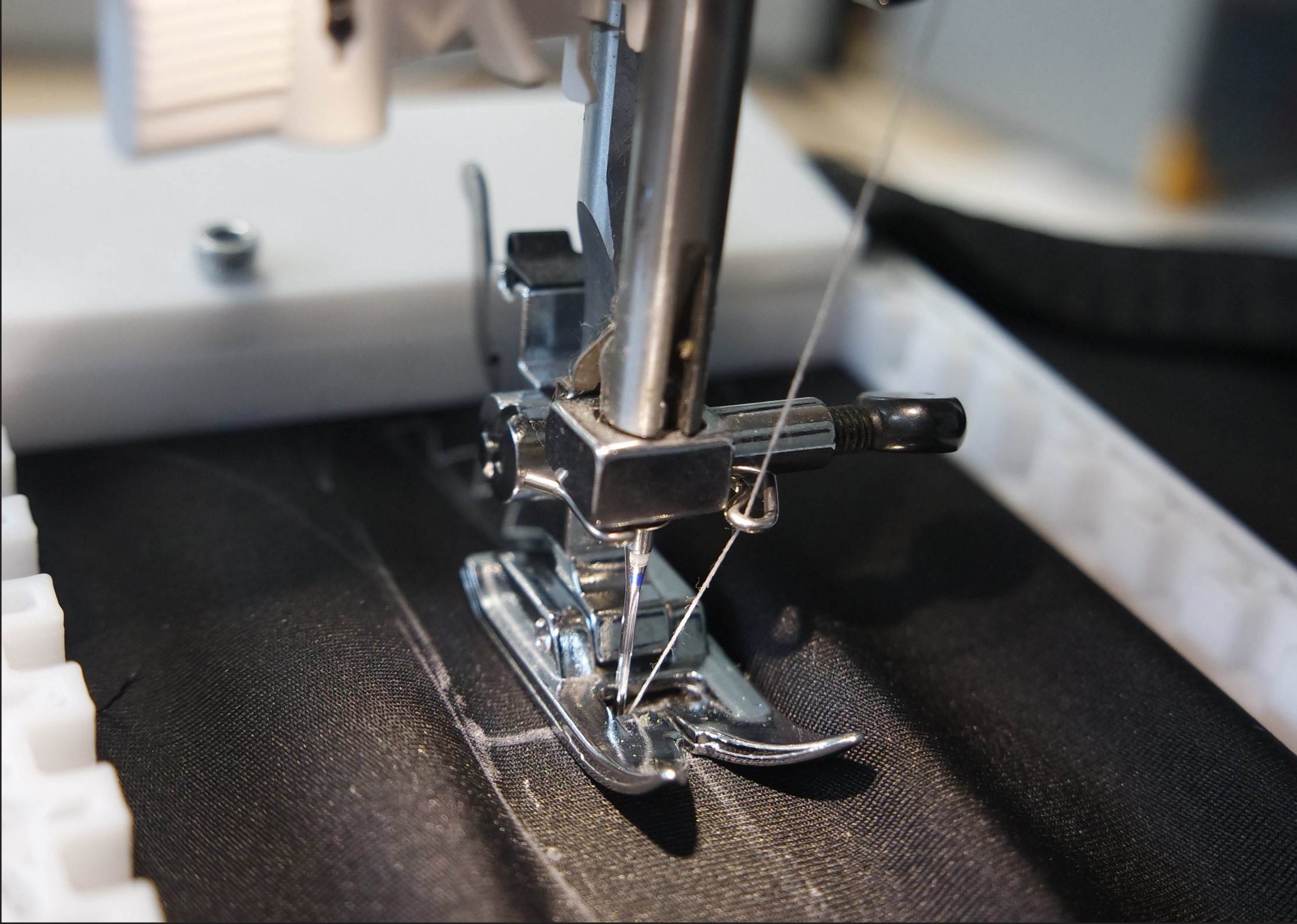
Figure 1 A snapshot of the manufacturing process of the knee sensor sleeve, where the sensor is sewn onto the fabric with preset parameters.
