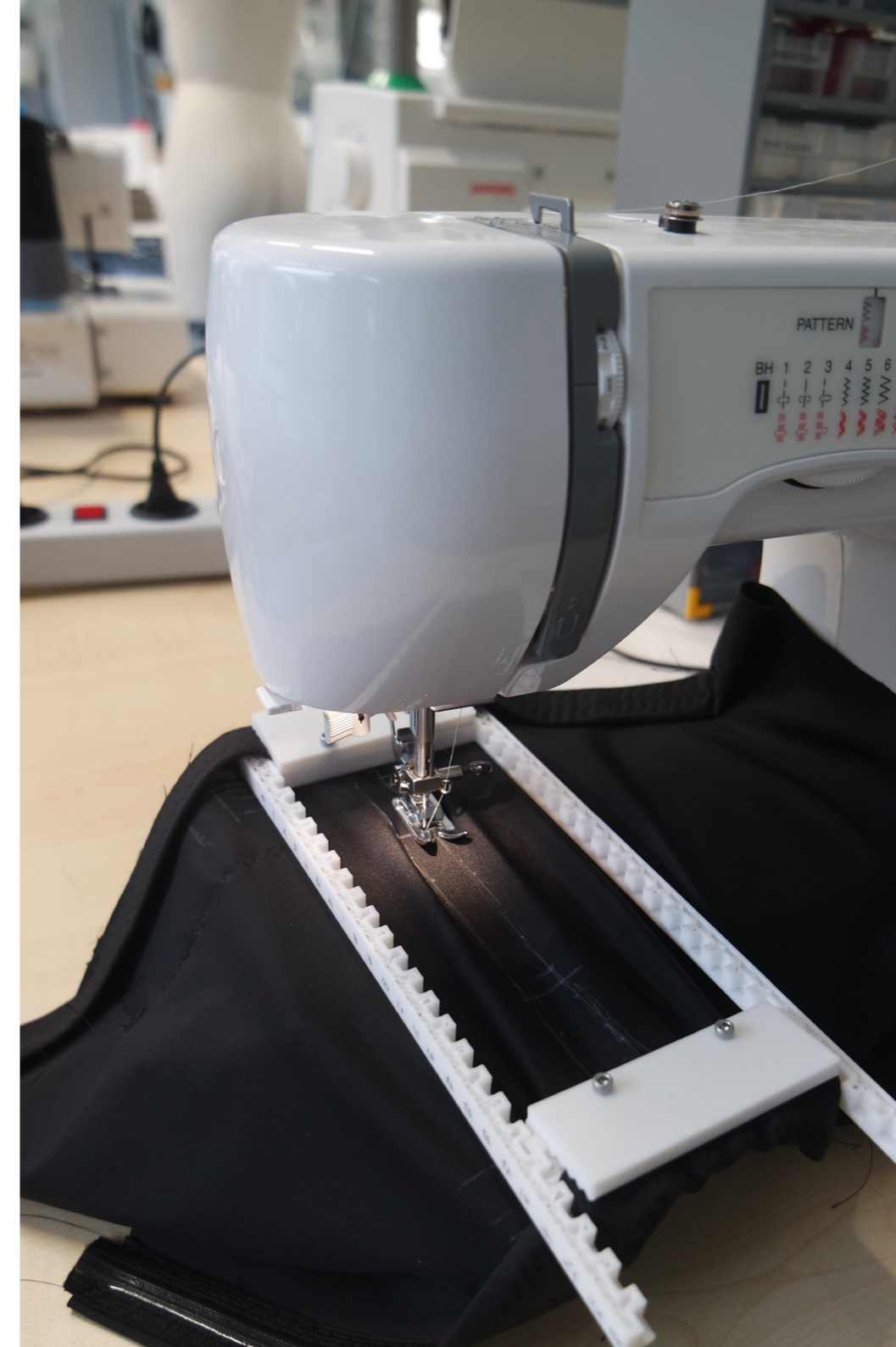
Figure 76. The sensor is stitched while being stretched using a stretch frame, which allows the fabric to be stretched to different extents.
