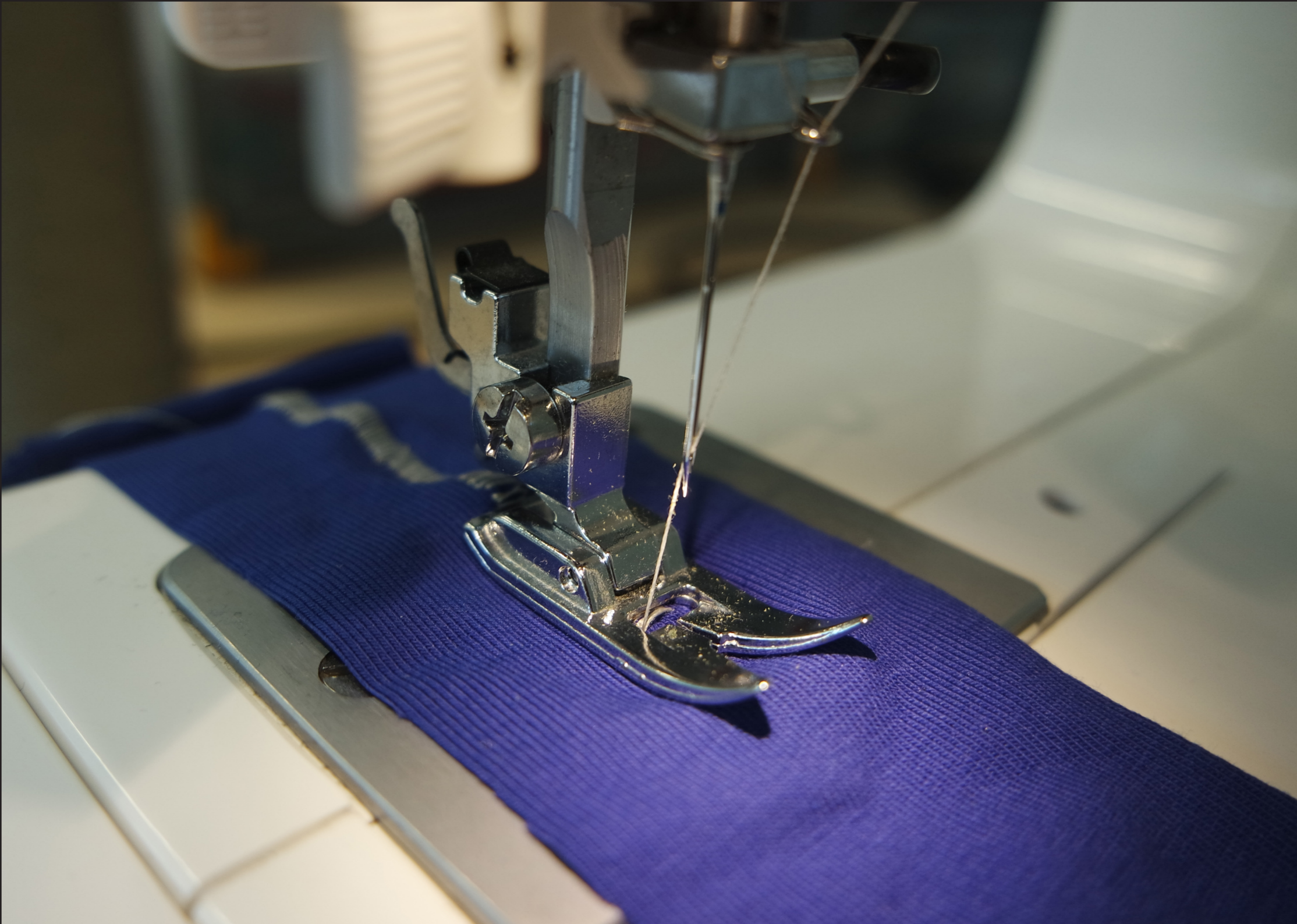
Figure 7 The manufacturing of a textile strain sensor, where the yarn is sewn onto the fabric with preset parameters.
