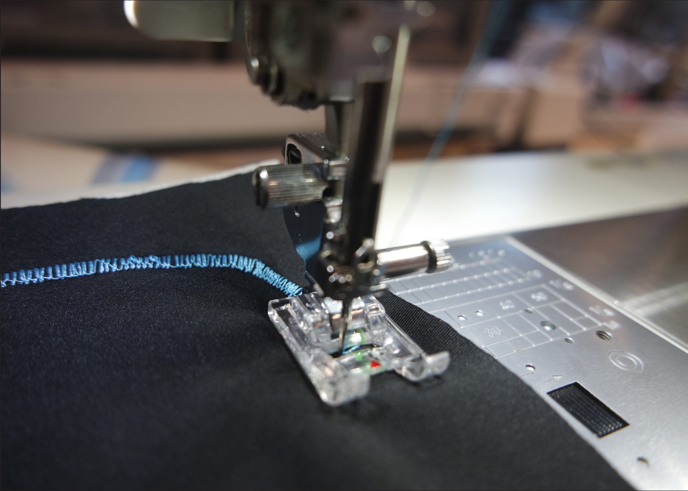
Figure 71. A snapshot of the manufacturing process of the knee sensor sleeve, where the design part of the sleeve is being embroidered
