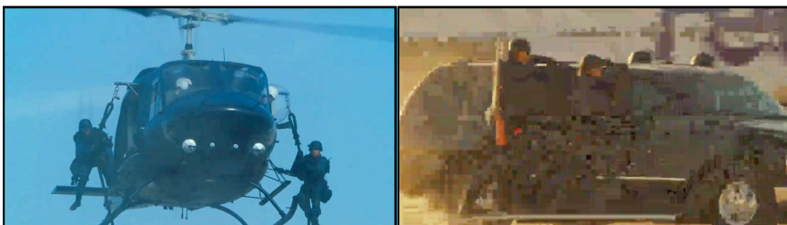
Figure 5.2. Video segments used for the experiment were taken from action movies and were chosen to have highly dynamic sequences. Varying the bitrate used to compress the videos from higher bitrates (left 1237 bit/s) to lower ones (right 209 bit/s) gave a wide range of quality for the generated videos.
