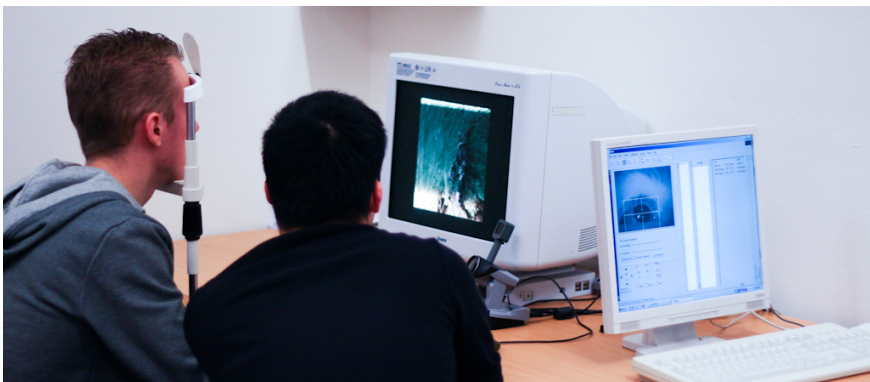
Figure 3.2. Participants place their head on a chin-rest positioned at a fixed distance from the display. The eye-tracker is positioned next to the display. The experimenter controls the eye tracker and runs the experiment using another monitor not visible to the participant.
