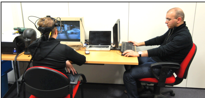
Figure 4.2. Experimental setup. The viewer watched the videos on a CRT monitor while wearing a head mounted eye tracking device. The experimenter ran the experiment from a non-intrusive position.
