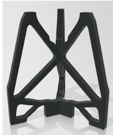
Figure 4.2: Design obtained after using the SOLIDWORKS application to transform the single arm design into a three-arm design
