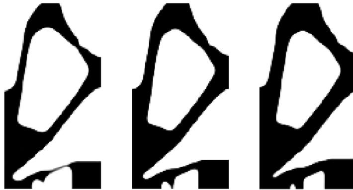
Figure C.5: Resulting eroded (left), intermediate (middle) and dilated (right) topologies from robust CM TO with hotspot constraint with an output displacement for the intermediate design  $u_{\text{out}} = 35.4$ .
