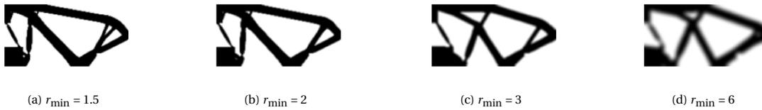
Figure 3.4: Generated designs with volume fraction  $f_0 = 0.4$  and varying filter radius  $r_{\min} = 1.5, 2, 3$  and  $6$
