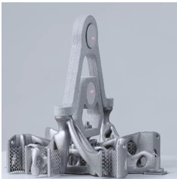
Figure 1.1: Metal compliant mechanism made by additive manufacturing [11]
