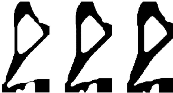
Figure B.5: Resulting eroded (left), intermediate (middle) and dilated (right) topologies from robust CM TO with hotspot constraint with an output displacement for the intermediate design  $u_{\text{out}} = 34.6$ .
