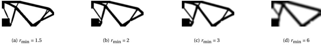
Figure 3.3: Generated designs with volume fraction  $f_0 = 0.3$  and varying filter radius  $r_{\min} = 1.5, 2, 3$  and  $6$
