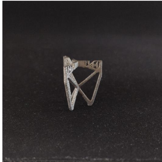
Figure 4.6: Smallest gripper in an upside down position to show the lack of material at the bottom of the gripper
