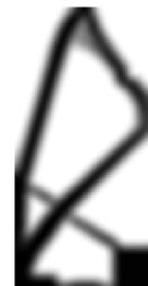
(d) Resulting topology from CM TO with hotspot constraint using  $T_{\text{crit}} = 1.7$  with resulting output displacement  $u_{\text{out}} = 30,5$
