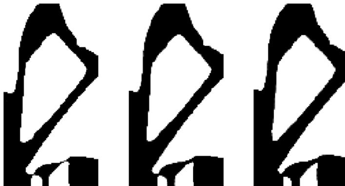
Figure B.1: Resulting eroded (left), intermediate (middle) and dilated (right) topologies from robust CM TO with hotspot constraint with an output displacement for the intermediate design  $u_{\text{out}} = 35.8$ .
