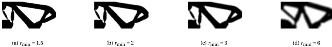
Figure 3.5: Generated designs with volume fraction  $f_0 = 0.5$  and varying filter radius  $r_{\min} = 1.5, 2, 3$  and  $6$
