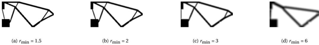
Figure 3.2: Generated designs with volume fraction  $f_0 = 0.2$  and varying filter radius  $r_{\min} = 1.5, 2, 3$  and  $6$
