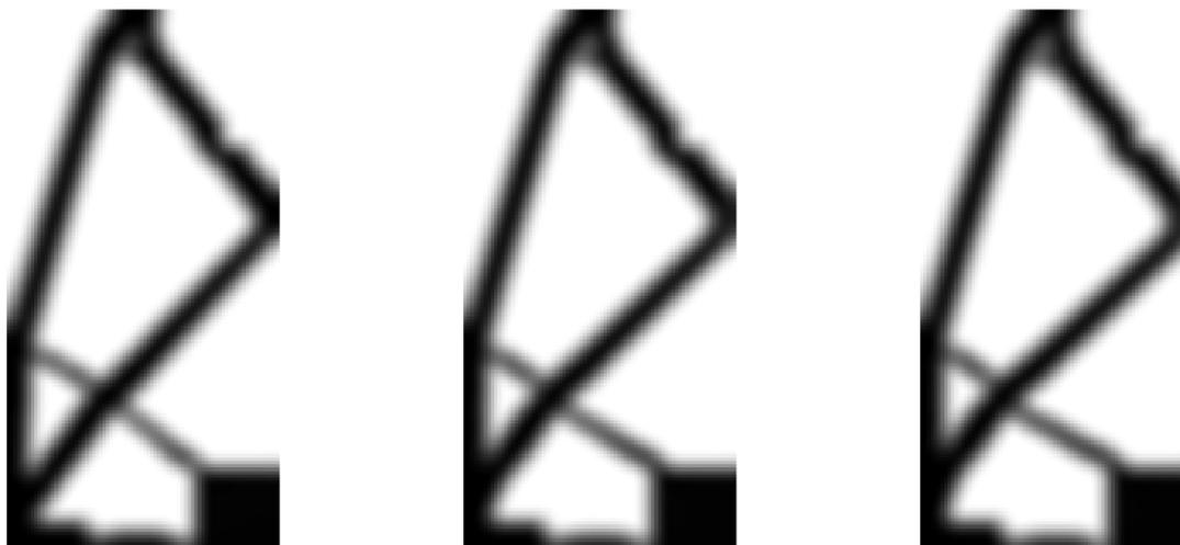
(a) Resulting topology from CM TO with hotspot constraint using thermal penalization factor  $r = 3$  with resulting output displacement  $u_{\text{out}} = 30,8$
