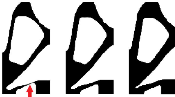
Figure 5.8: Resulting eroded (left), intermediate (middle) and dilated (right) topologies from robust CM TO without hotspot constraint with an output displacement for the intermediate design  $u_{\text{out}} = 35.5$ . The red arrow indicates a very thin member of the eroded design
