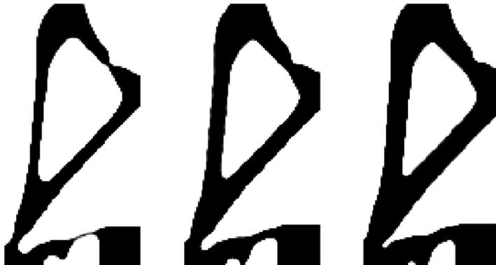
Figure C.1: Resulting eroded (left), intermediate (middle) and dilated (right) topologies from robust CM TO with hotspot constraint with an output displacement for the intermediate design  $u_{\text{out}} = 35.1$ .
