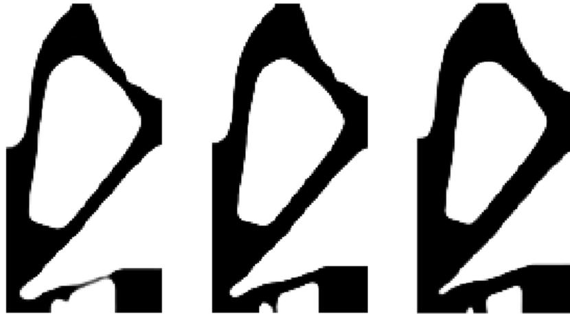
Figure 5.23: Resulting eroded (left), intermediate (middle) and dilated (right) topologies from robust CM TO with hotspot constraint with the base plate on the south side of the design and using a slab thickness  $s = 24$ , with an output displacement for the intermediate design  $u_{out} = 35.3$
