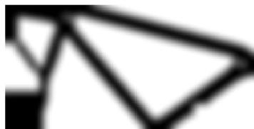
Figure 3.6: Final chosen design obtained with topology optimization with filter radius  $r_{\min} = 6$ , volume fraction  $f_0 = 0.3$  and objective value  $32.0211$
