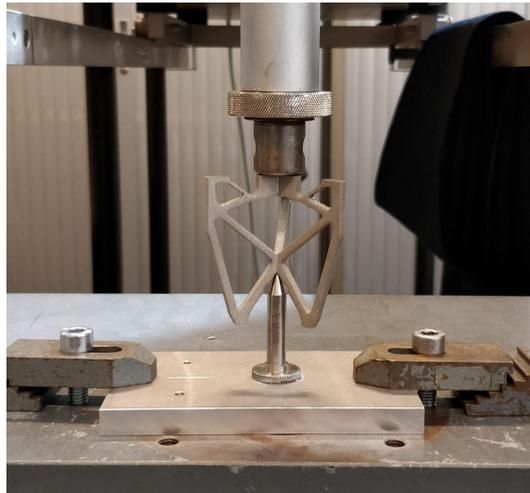
Figure 4.7: Mechanical test setup of the triple size gripper in the upside down position constraint using a pin. A downward force is applied on the bottom of the gripper
