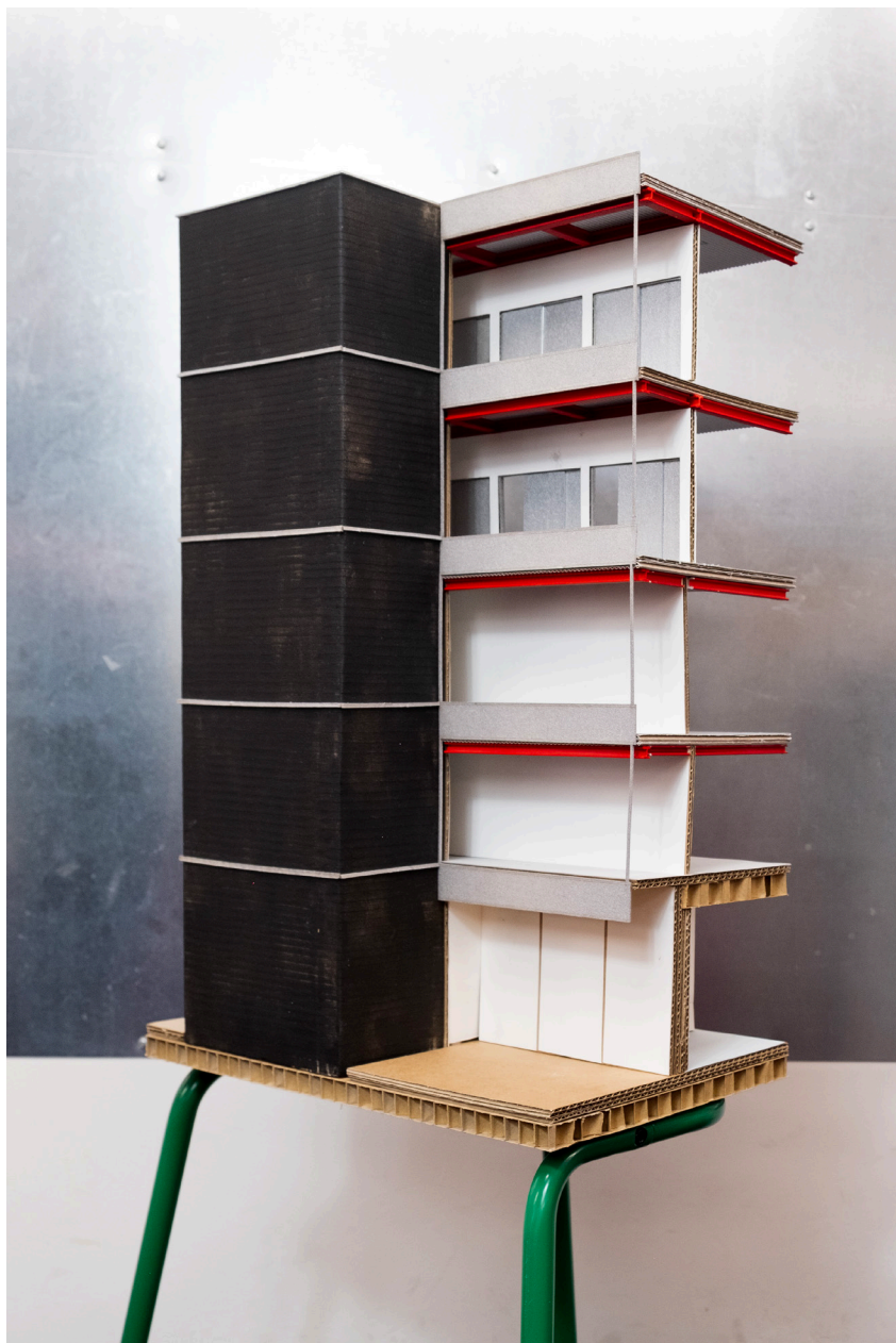
Fig.171 1:33 model emphasizing the exposed lintel/tie-beams
