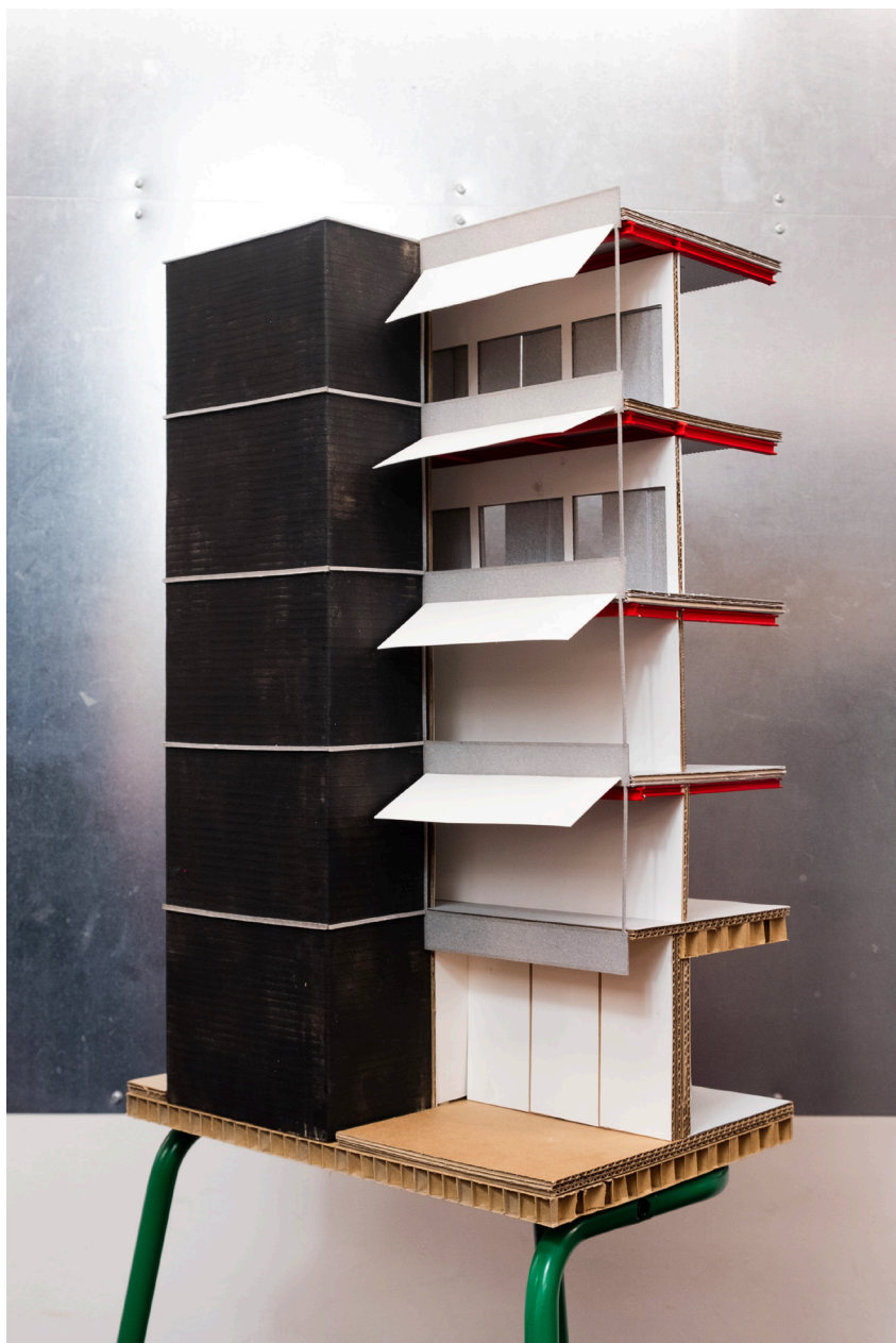
Fig.170 1:33 model with sun-shading system of the south facade
