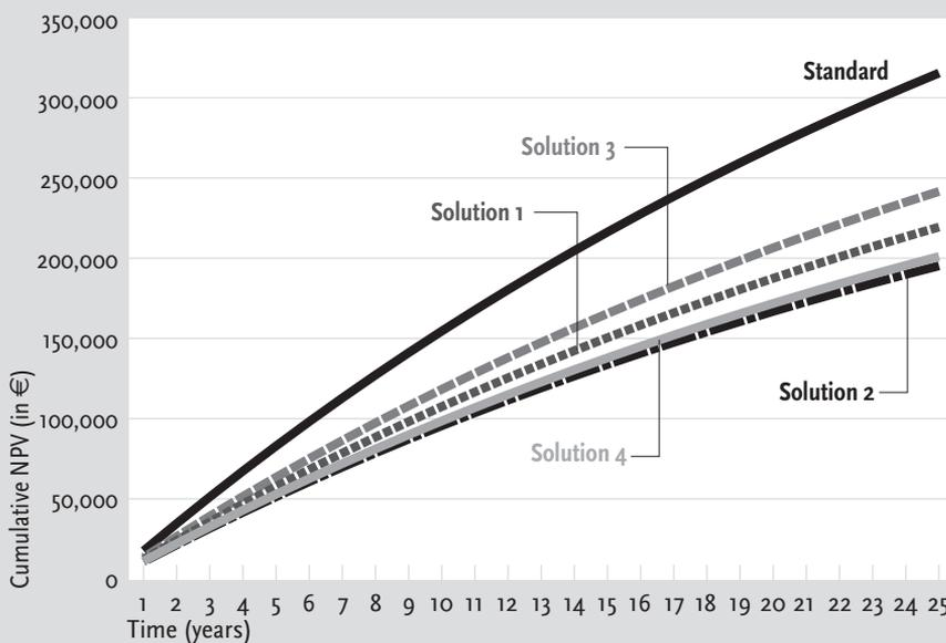
The comparison between standard and energy-efficient renovations shows that Solution 2 can save 38% more in total energy costs and reduce CO<sub>2</sub> by 70% more than a standard renovation. Solution 4 would result in an extra reduction of 36,021 kg (75%) in CO<sub>2</sub> emissions compared with the 'zero
