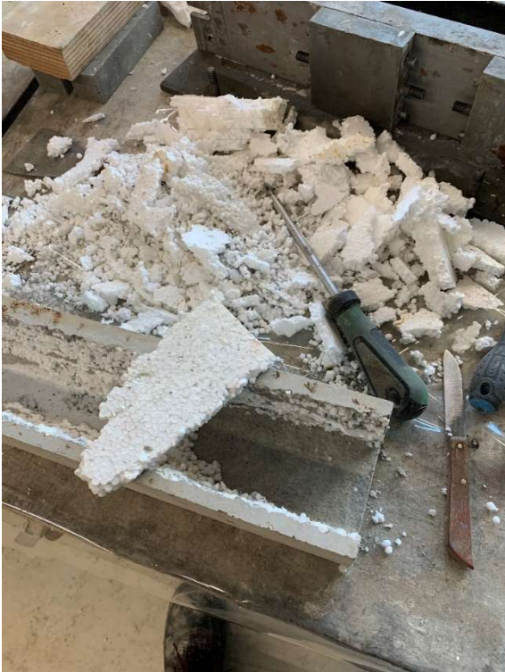
Appendix figure 67: demoulding of an SHCC U-shape with Styrofoam as the inside mould
