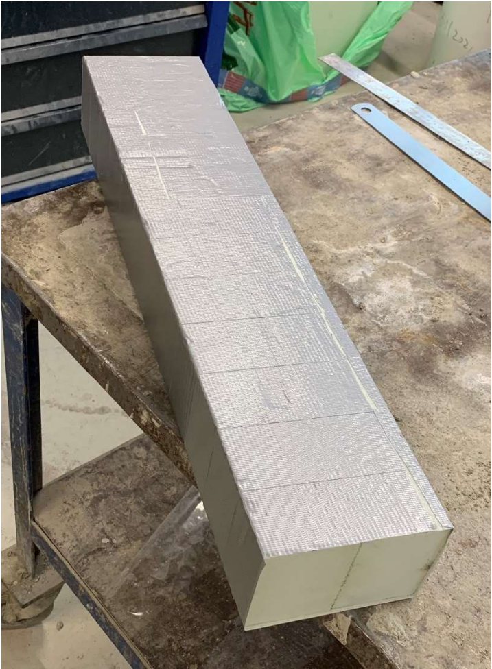
Appendix figure 71: inside Styrofoam mould wrapped in tape
