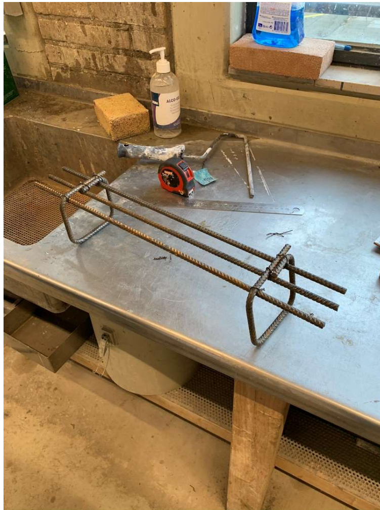
Appendix figure 69: prepared reinforcement for medium scale experiment
