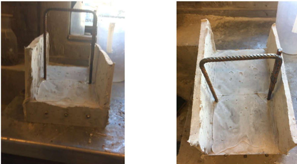
Figure 1-5: concept of a U-shaped SHCC mould as proposed by (Huang, 2017)
