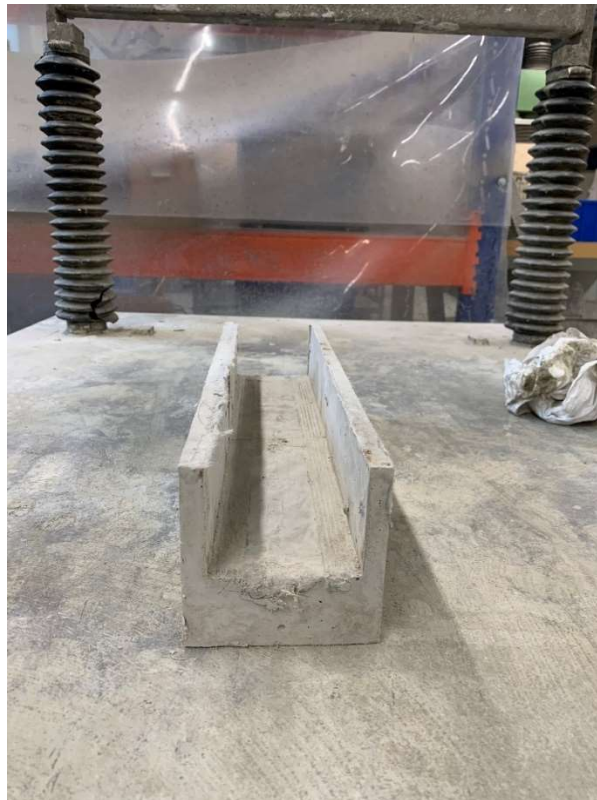
Appendix figure 65: U-shape made out of the correct SHCC mixture
