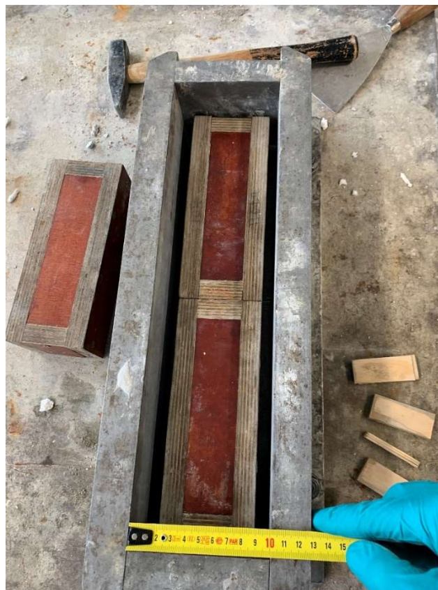
Figure 2-4: inside and outside moulds for casting a U-shaped mould
