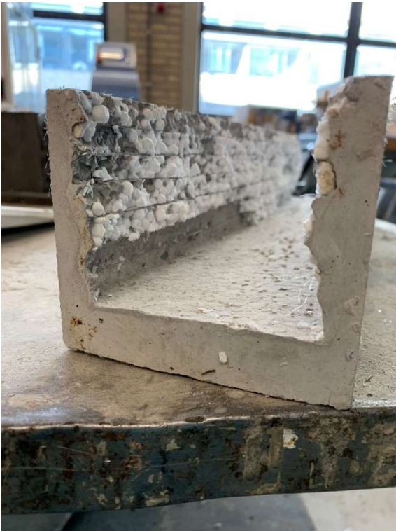
Appendix figure 68: the effect of Styrofoam plates on the demoulding process
