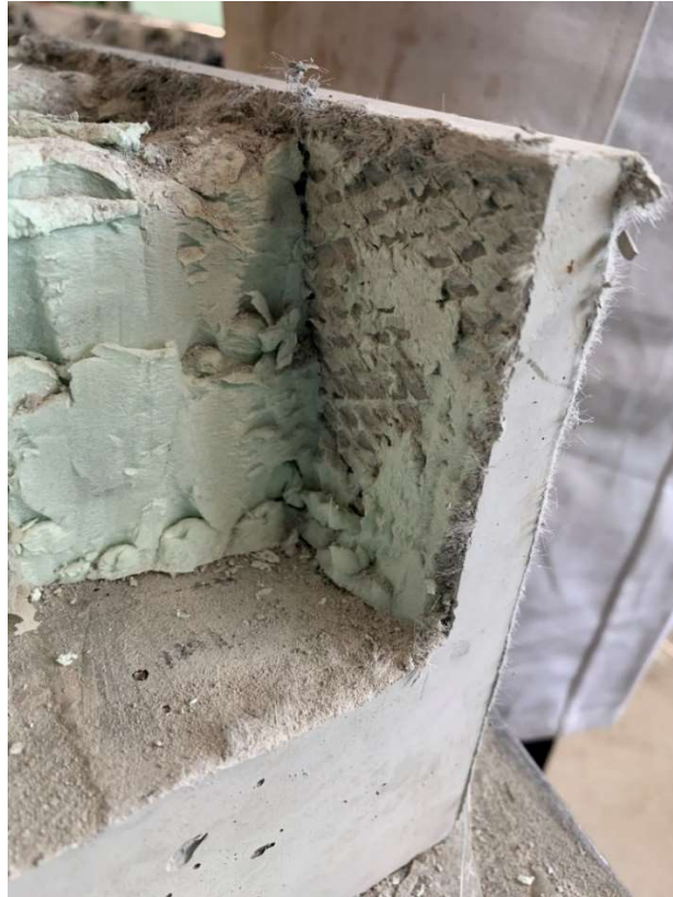
Appendix figure 70: Styrofoam sticking to the SHCC
