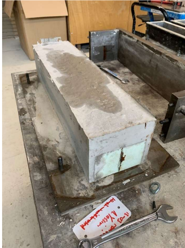
Figure 2-5: inverse U-shape after casting
