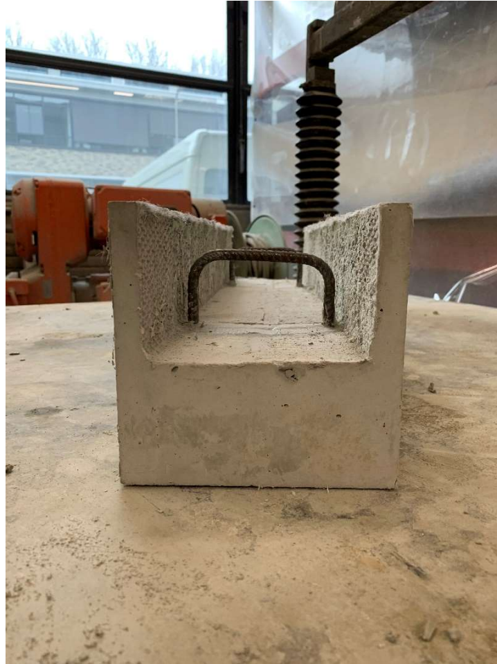
Figure 2-9: end result after demoulding a reinforced U-shaped SHCC mould
