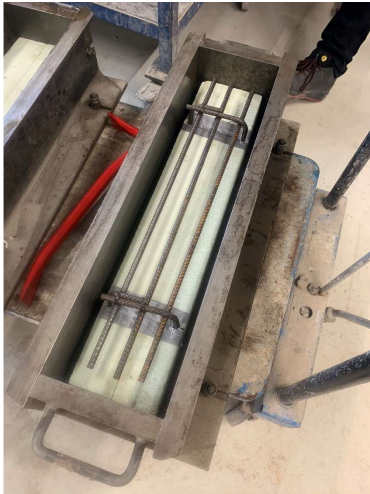
Figure 2-8: preparation of a U-shaped SHCC mould with steel reinforcement in it
