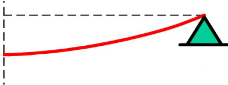
Appendix figure 56: deflection of half a span for a simply supported beam (Welleman, 2018)
