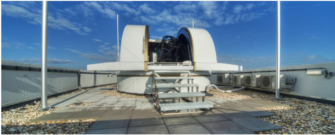
Figure 1.3: TNO optical ground station with an 80 cm Ritchey-Chrétien alt-az telescope 5 .
