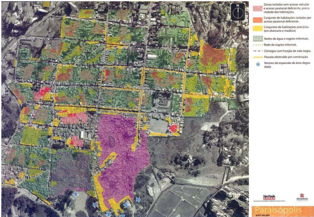
Figure 2: risk map of sewerage connection and accessibility.
