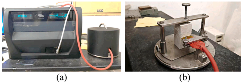
Fig. 4. Thermal conductivity test. (a) Hot Disk device; (b) Placement of samples.
