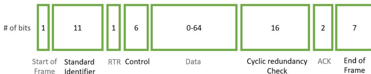
Figure 11.4: The CAN data frame message fields
