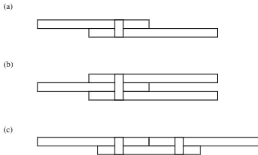
Figure 38: Different types of mechanical joints: (a) single lap, (b) double lap, (c) butt [2]
