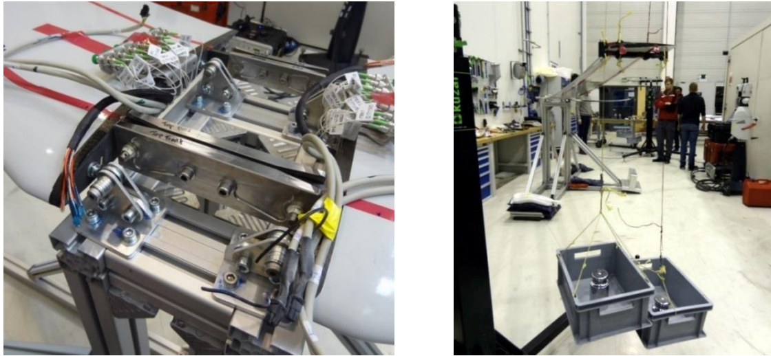
Figure 12: Attachment of reference wing to the test-stand (left), load-application for the static tests (right)
