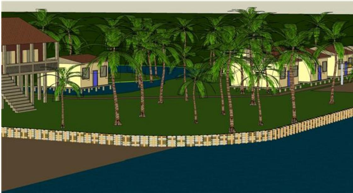
Figure 4.28: Sandbags with bamboo poles
