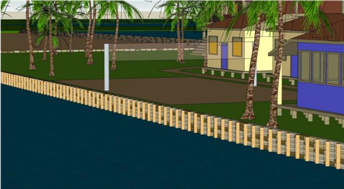
Figure 4.29: Sandbags with bamboo poles
