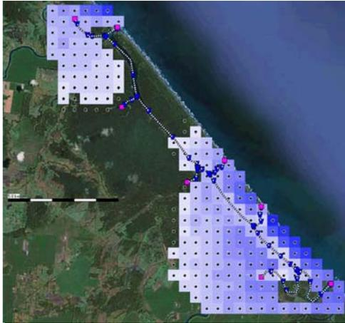
Figure 3.30: 2D screenshot inundation; peak discharge of 2000 m<sup>3</sup>/s
