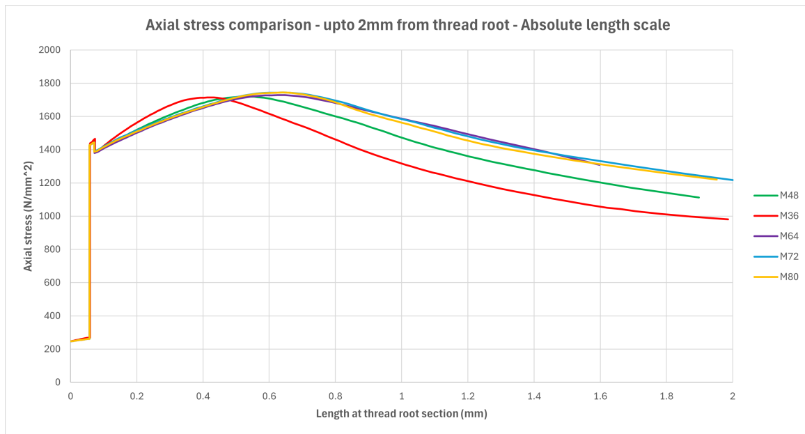
Figure 6.14: Axial stress plots up to 2mm from the critical thread root section edge
