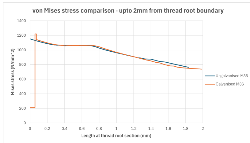
Figure 4.25: Mises stress up to 2mm depth from the thread root boundary. Notice the zeta and delta layer values (first two plateaus) have attained ultimate tensile strength as seen in figure 4.6
