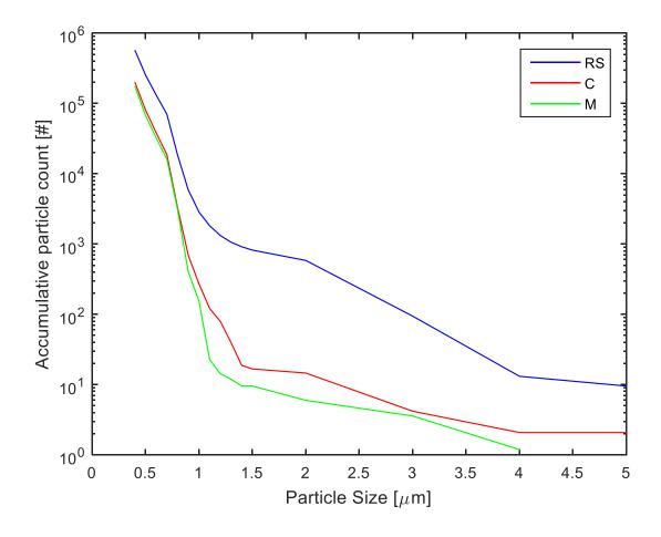
Figure 3.2. Particles counts between 0.4 and 5.0  $\mu$ m of raw sewage after settling (RS) and after chemically enhanced settling with flocculant (C) and coagulants (M).
