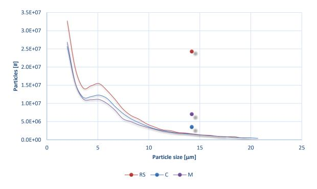
Figure 2.5. Particle count of the digested flocculated sludges (C and M) and the digested reference sludge (RS).
