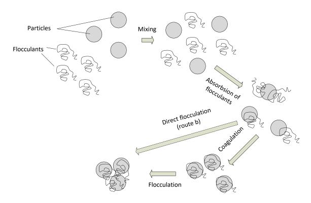
Figure 1.6. Processes involved in flocculation of particles. Adapted from Gregory (1988).
