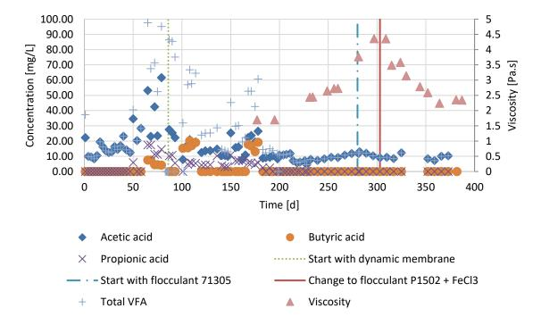
Figure 4.3. VFA concentrations of the reactor and viscosity of the reactor operated as conventional anaerobic digester in period 1 (day 1 - 86), operated as an AnDMBR in period 2 (day 86 - 303) and operated as an AnDMBR with flocculation aid addition in period 3 (day 303 - 386).
