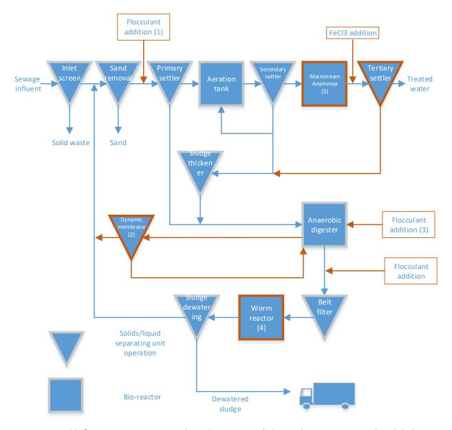
Figure 6.1. Possible future sewage treatment plant where primary sludge production is maximized, and sludge production and footprint are minimized. Possible applications of flocculant additions are indicated. The numbers 1-5 are further discussed in the text below.
