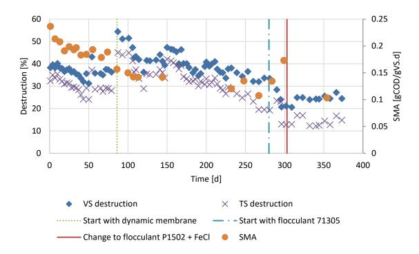
Figure 4.2. TS and VS destruction and SMA of the reactor operated as conventional anaerobic digester in period 1 (day 1 - 86), operated as an AnDMBR in period 2 (day 86 - 303) and operated as an AnDMBR with flocculant addition in period 3 (day 303 - 386).
