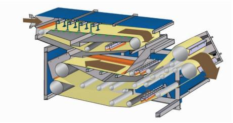
Figure 1.10. Dewatering centrifuge (top, source www.alfalaval.com). Sludge is fed on the right, dewater sludge leaves the centrifuge on the right, liquid leaves the centrifuge on the left. Belt press (bottom, source: frcsystems.com) presses sludge between two belts that are tightened over course of the path through the machine.
