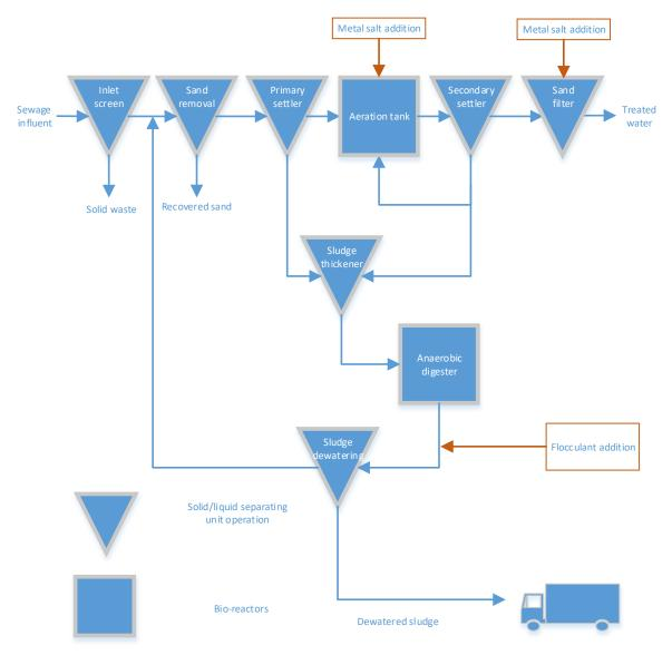
Figure 1.8. Schematic overview of a typical sewage treatment plant with biological and chemical nutrient removal.
