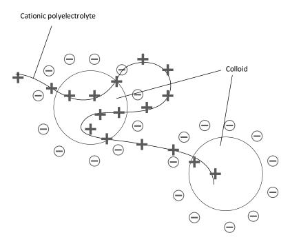
Figure 1.4. Polymer bridging of cationic polyelectrolyte between two negatively charged colloids.
