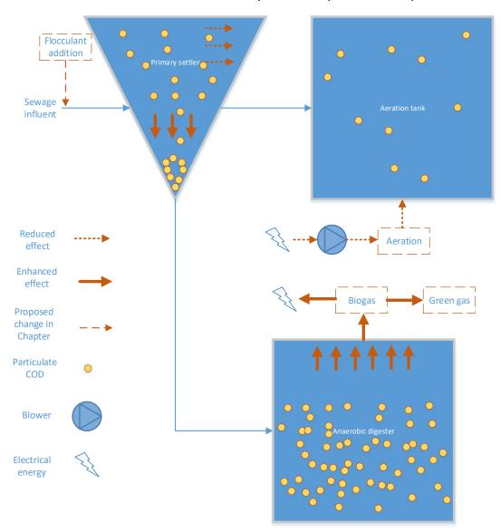
Figure 1.12. Schematic overview of possible benefits of applying chemically enhanced primary treatment: more particulate COD is directed to the anaerobic digester instead of the aeration tank, yielding more biogas and a reduced electrical energy consumption for aeration.
