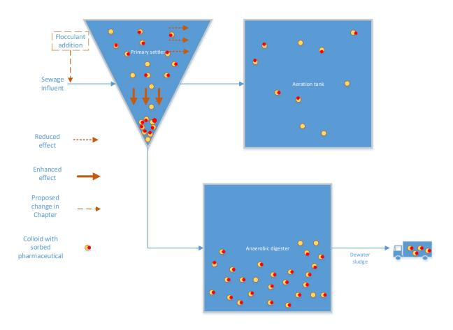
Figure 1.13. Schematic overview of possible benefits of applying chemically enhanced primary treatment: more colloidal bound pharmaceuticals are directed to the smaller sludge stream to facilitate treatment and/or disposal after sludge dewatering.
