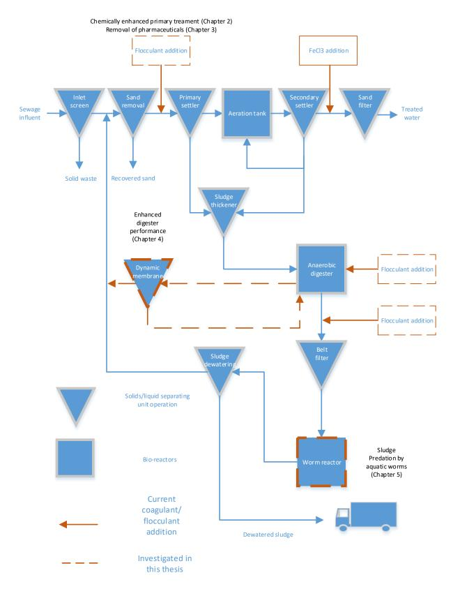
Figure 1.11. Overview of novel flocculant applications investigated in this thesis.
