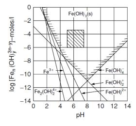
Figure 1.2. Equilibrium solubility products of iron hydroxides in water as function of the pH. The dashed area is the working area in wastewater treatment. Adapted from Bratby (2006).
