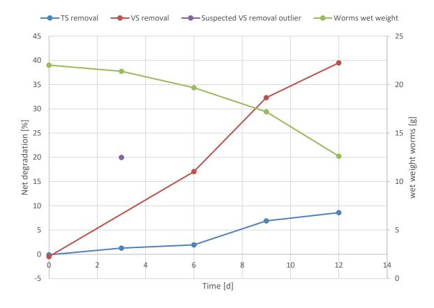
Figure 5.2. Degradation of TS, VS and the quantity of worms in the 12 day experiment
