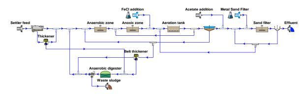
Figure 2.6. Biowin print-out representing a schematic overview of the STP Leiden Noord including CEPT combined with anaerobic digestion of excess sludge (150.000 P.E.).
