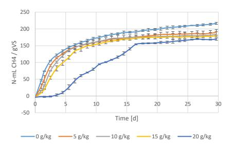
Figure 4.5. BMP tests of WAS with different flocculant concentrations. Increased flocculant concentration decreases the BMP values.
