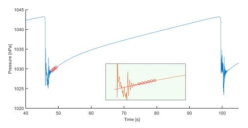
Figure 9.4. Example of pressure built-up during pressure equalization between the gas collector of the reactor and the gas phase of first tube of the gas flow meter at a flow of 5 N-L/h. The extrapolation (in red) is used to estimate the pressure built-up during the click from which the gas flow during the click can be estimated.
