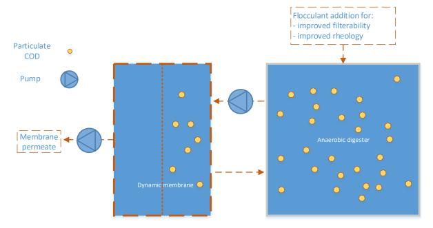
Figure 1.14. Schematic overview of setup where a dynamic membrane is applied to uncouple the hydraulic retention time and solids retention time. Flocculants can be added to improve the filterability and the rheology in the anaerobic digester.
