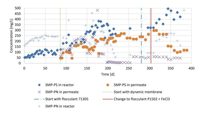
Figure 4.6. Concentrations of SMP-PS (polysaccharides) and SMP-PN (polypeptides) in the supernatant and the permeate of the reactor operated as conventional anaerobic digester in period 1 (day 1 - 86), operated as an AnDMBR in period 2 (day 86 - 303) and operated as an AnDMBR with flocculant addition in period 3 (day 303 - 386).
