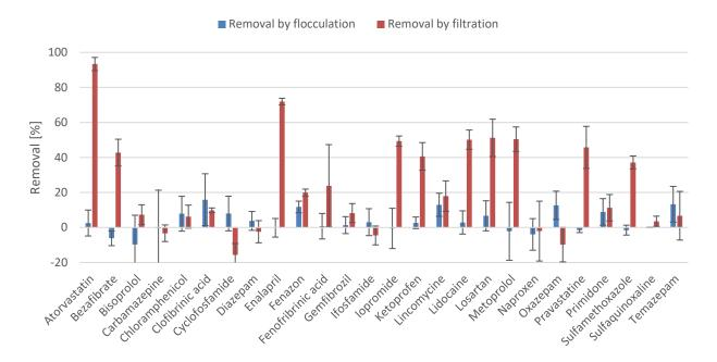
Figure 3.3. Removal efficiencies of pharmaceuticals when removing humic substances by flocculation and ultra-filtration. When using ultra-filtration, significant removal can be observed of pharmaceuticals, often leading to the erroneous conclusion that pharmaceuticals are attached to colloids.
