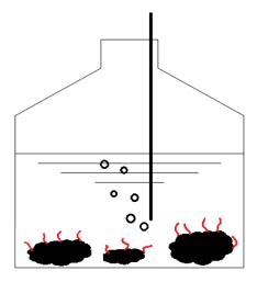
Figure 5.1. Schematic representation of bottle experiment. Flocculated sludge (black mass) accumulated on the bottom of the flask. The worms waved their tail through the water for oxygen uptake. The flocculated sludge solids remained separated from the liquid over the course of the 12 d experiment. Aeration is performed at approximately 15 cm above the sludge bed to prevent shear stress.
