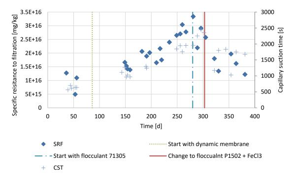
Figure 4.4. The specific resistance to filtration (SRF) and the capillary suction time (CST) of the effluent sludge of the reactor operated as conventional anaerobic digester in period 1 (day 1 - 86), operated as an AnDMBR in period 2 (day 86 - 303) and operated as an AnDMBR with flocculation aid addition in period 3 (day 303 - 386).
