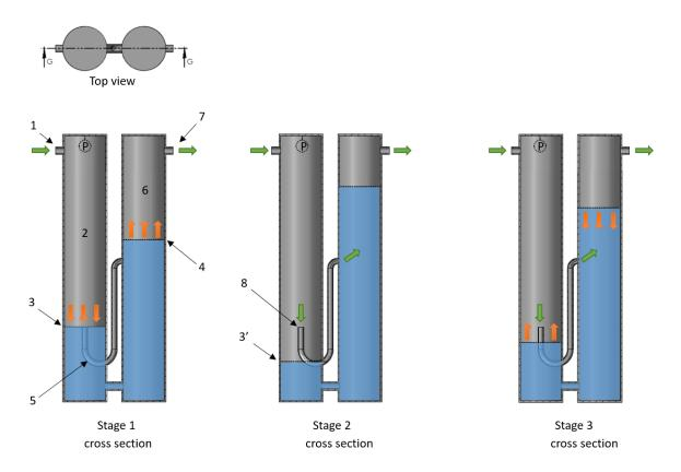
Figure 9.2. Schematic overview of physical functioning of the gas flow meter equipped with a pressure sensor (P) coupled to an Arduino Uno micro controller. All stages are cross sections of the device at line 'G' of the top view. The green arrows represent the gas flow and the orange arrows represent the water movement.
