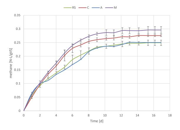
Figure 2.1. Methane production during the BMP (BMP\_1) test in N-mL methane per g VS substrate of primary sludges of the CEPT Experiment. C refers to sludge produced from sewage influent with 10 ppm cationic flocculation aid (FA); A refers sludge produced by with 10 ppm anionic FA; and M refers to sludge produced with 10 ppm organic coagulant and 2 ppm cationic FA. RS is the reference situation where sludge was produced by plain settling without FA additions.
