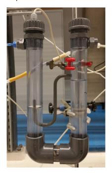
Figure 9.1. Photo of the gas flow meter used in this study. The gas flow meter is made of 40 mm PVC piping.
