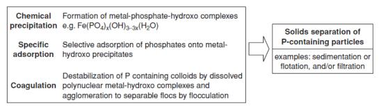
Figure 1.1. Summary of phosphorus removal from wastewater by using metal salt addition. Scheme adapted from Bratby (2006).
