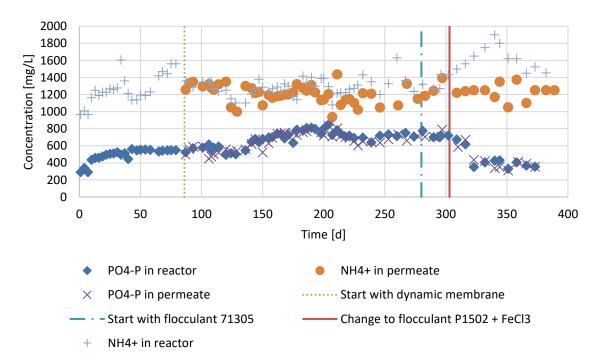
Figure 4.7. Ortho-phosphate (PO4-P) and ammonium (NH4+) concentrations of the reactor operated as conventional anaerobic digester in period 1 (day 1 - 86), operated as an AnDMBR in period 2 (day 86 - 303) and operated as an AnDMBR with flocculant addition in period 3 (day 303 - 386).
