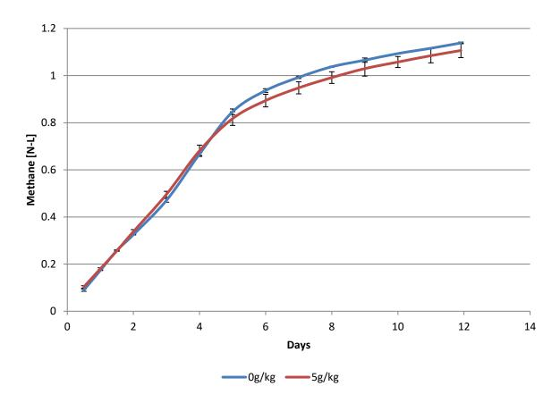
Figure 2.4. BMP test with non-stirred conditions (BMP\_3\_Unstirred) with flocculated sludge (5 g kg<sup>-1</sup>) and non-flocculated sludge (0 g kg<sup>-1</sup>).
