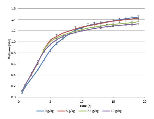
Figure 2.2. Methane production during a BMP test with primary, secondary sludge as substrate.  $C_{FA}$  was added directly to the BMP test bottles at t=0 in different concentrations (BMP\_2\_ $C_{FA}$ ). All samples contained the same amount and type of primary and secondary sludges.
