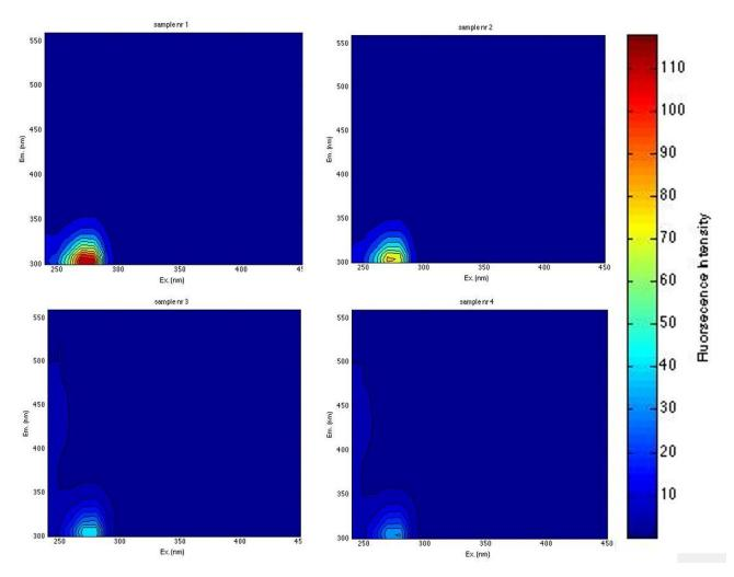
Figure 2.3. F-EEM images of the supernatant of BMP\_2\_ $C_{FA}$  on day 7 with 0 g kg<sup>-1</sup> (sample nr. 1), 5 g kg<sup>-1</sup> (sample nr. 2), 7.5 g kg<sup>-1</sup> (sample nr. 3) and 10 g kg<sup>-1</sup> (sample nr. 4). On 275 nm (Ex.) and 310 nm (Em.) is the area where fluorescence of tryptophan, characterising microbial derived proteins, is located. The higher the density in this area, the more microbially derived protein is present.
