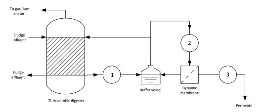
Figure 4.1. Schematic overview of the AnDMBR setup used. The first pump (1) transports the sludge to the buffer vessel from which it is circulated over the membrane by pump 2. The permeate pump (3) creates the pressure difference over the membrane by removing permeate.
