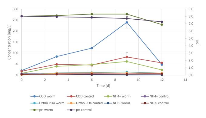
Figure 5.3. Development of concentrations and pH of the experiment with worms (worm) and the endogenous respiration (control).
