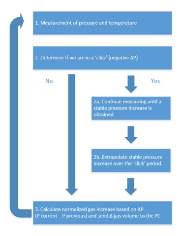
Figure 9.3. Schematic representation of the software loop that is executed in the Arduino Uno to measure the gas flow.
