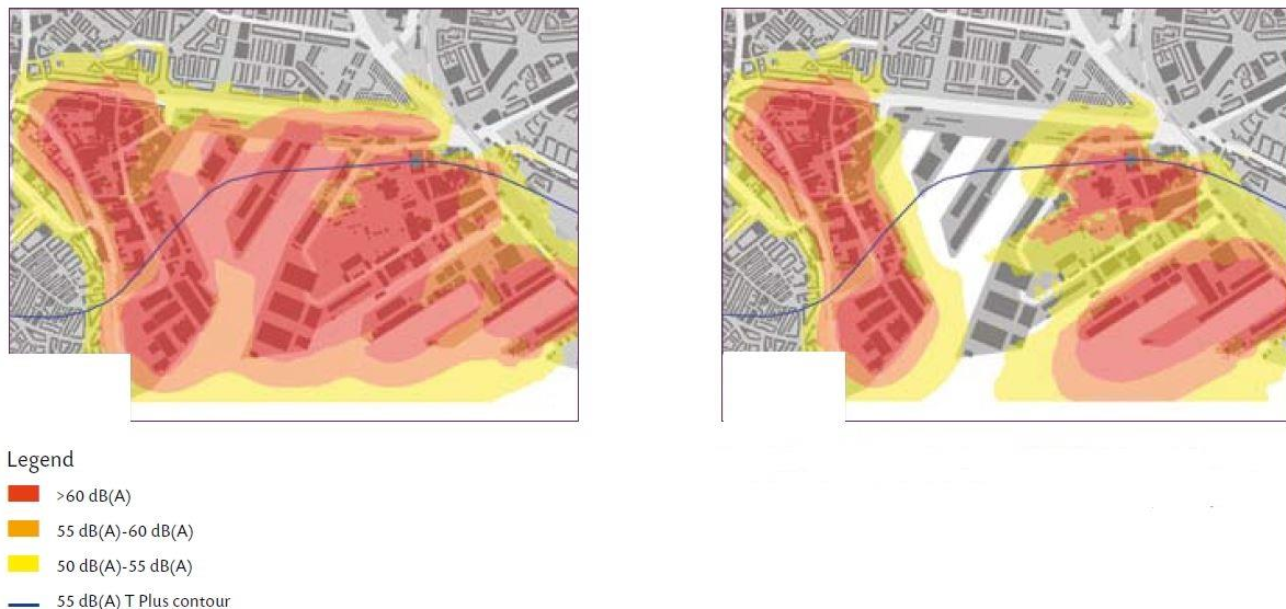
Figure 74: Sound analysis Merwe-Vierhavens. Left is the situation in 2007 and right is the current situation with some industrial harbour removed. (Projectbureau Stadshavens Rotterdam, 2009)
