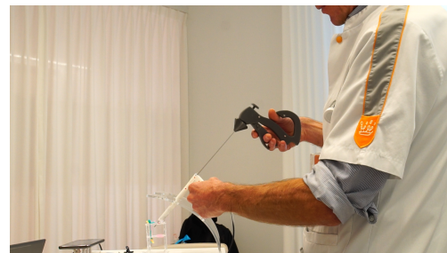
Figure 3: Still from the user test showing the markers (red dots on the white endoscope)
