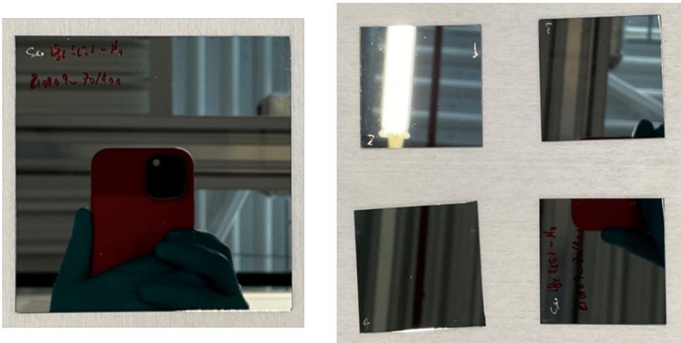
Figure 3.1: Mo on SLG substrate. a. 10x10cm 2 SLG/Mo substrate. b. 5x5cm 2 Four quadrant division.
