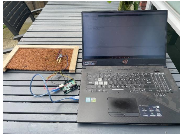
Figure 4.2: Testing the moisture sensor (Own work)
