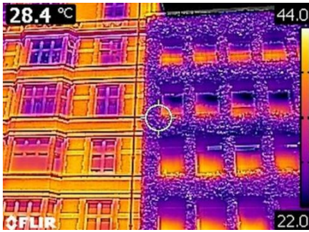
Figure 2.3: Infrared image of a living wall (Grant,2018)
