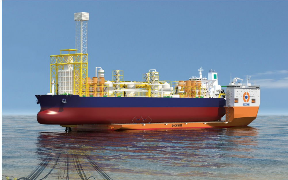
FIGURE 1.1: Vanguard with an FPSO loaded on deck[1]
