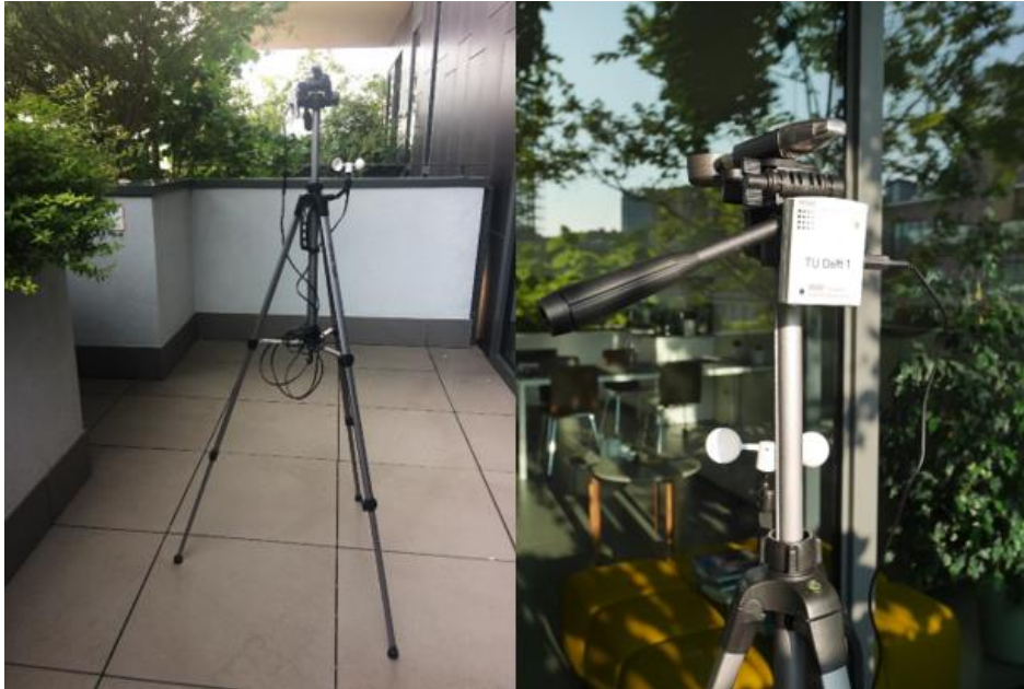
Figure 50: Setup of solar radiation, temperature/humidity and wind meters on balcony
