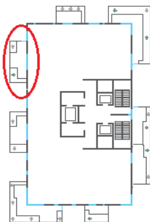
Figure 76: Typical balcony geometry of Bosco Verticale
