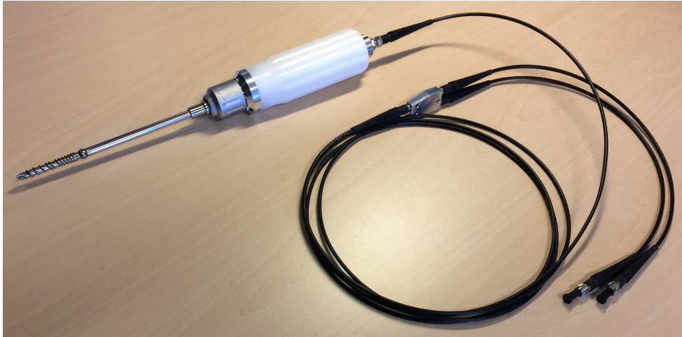
Figure 5.1: A depiction of the integrated pedicle screw and screwdriver used in the study, equipped with two optical fibers at the tip of the screw with a fiber distance of 1.22 mm.
