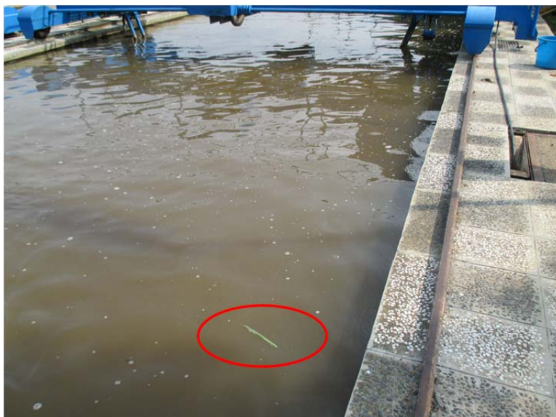
Figure 1. 15 Flowing Visual Object for Measuring 1-D Flow Velocity in Presedimentation Tanks
