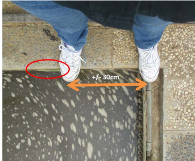
Figure 1.16 Approximation of Finishing Point of 1-D Flow Velocity in Presedimentation Tanks
