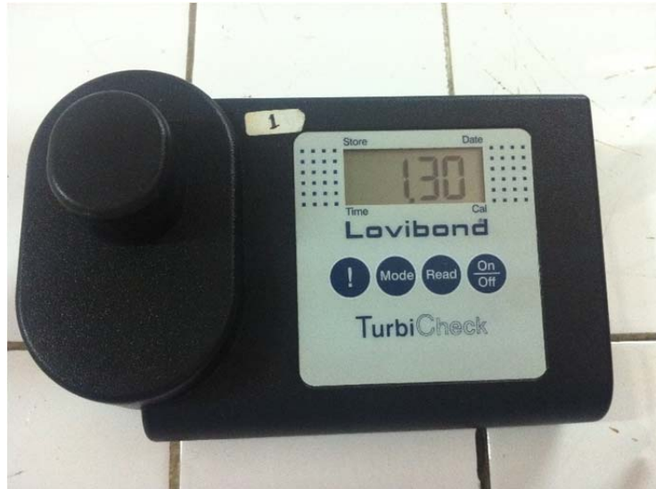
Figure 3. 13 Turbidity-meter used for turbidity measurements
