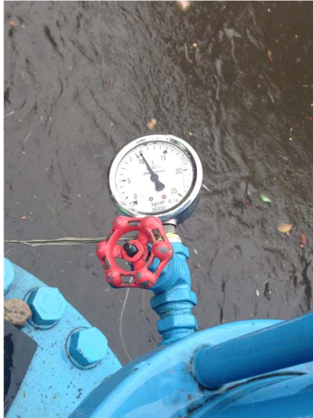
Figure 2. 3 Monthly pressure measurements conducted with a manometer
