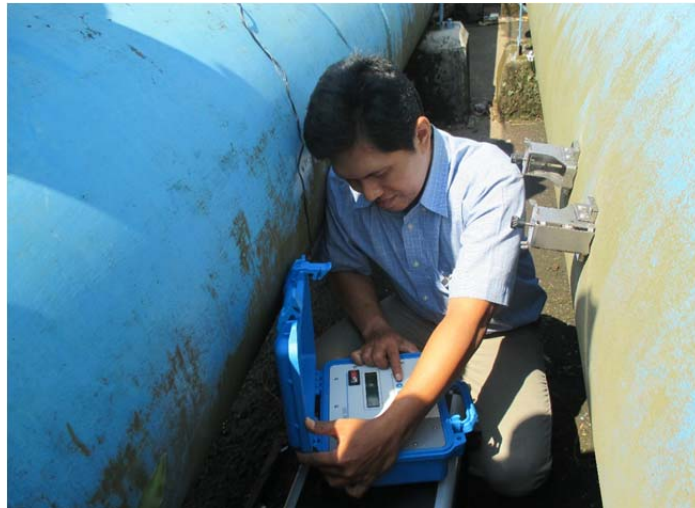
Figure 2. 14 Ultrasonic Flowmeter Measurement
