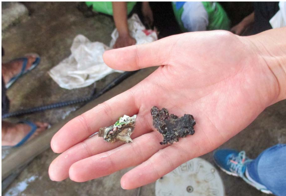
Figure 2. 13 Solids removed from the air valve causing the flooding
