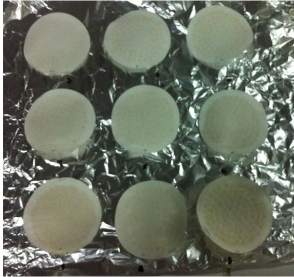
Figure 3. 15 Filters used for TSS analysis
