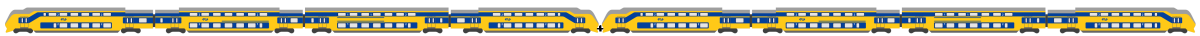
Figure 1.4: Rolling stock combination operating on the Dutch network, consisting of two rolling units of type VIRM4, each consisting of four carriages (Treinposities.nl, 2020).
