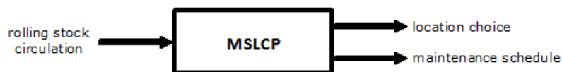
Figure 1: The characterizing input and output of the MSLCP : using a rolling stock circulation, an optimal maintenance location choice and an optimal maintenance schedule are determined.
