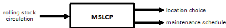
Figure 3.1: The characterizing input and output of the MSLCP : using a rolling stock circulation, an optimal maintenance location choice and an optimal maintenance schedule is to be determined. It must be noted that in addition, also the set of maintenance locations and the set of maintenance types needs to be provided as an input, but these have more the nature of a user setting and are therefore not provided in the current figure.
